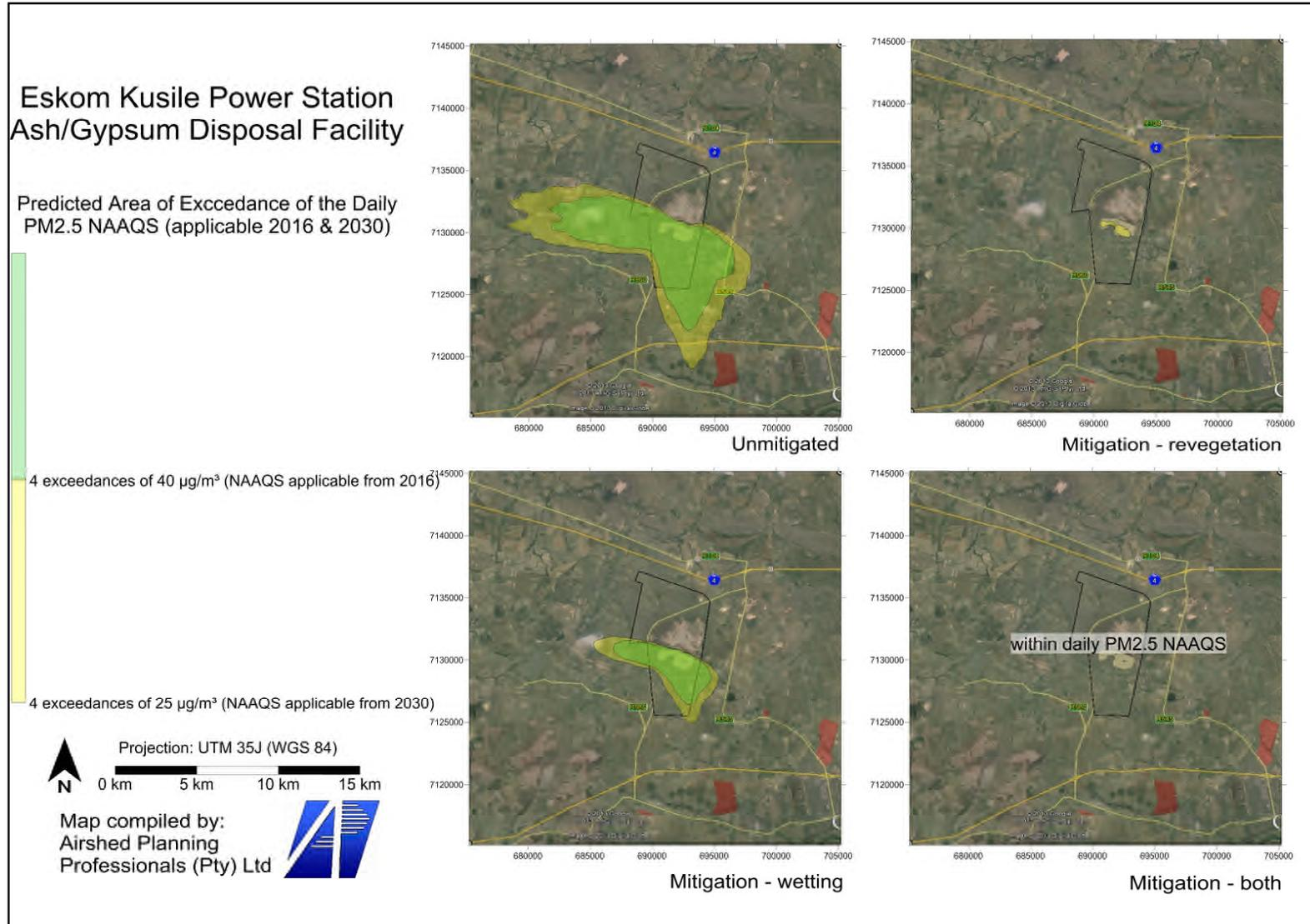
Figure 5-4: Predicted area of exceedance of the daily PM<sub>2.5</sub> NAAQS due to the disposal facility at Kusile Power Station
