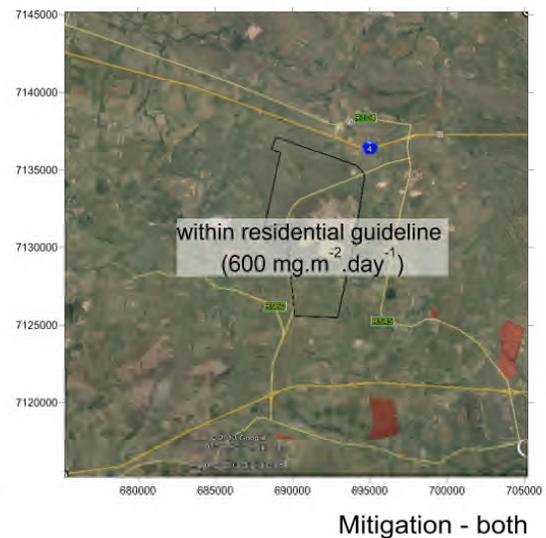
Figure 5-1: Predicted maximum monthly dust deposition as a result of windblown dust from the disposal facility at the Kusile Power Station
