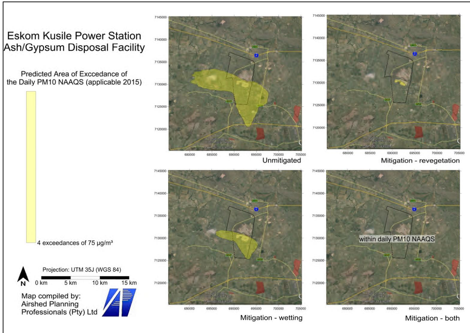
Figure 5-2: Predicted area of exceedance of the daily PM<sub>10</sub> NAAQS due to the disposal facility at Kusile Power Station
