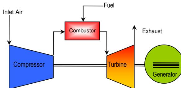
**Figure 2.2 Schematic of a process that a gas turbine undergoes in order to produce electricity.**
