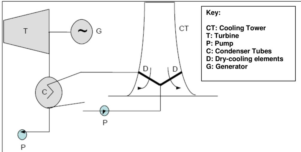
**Figure 2.5** Showing an indirect dry cooling system
