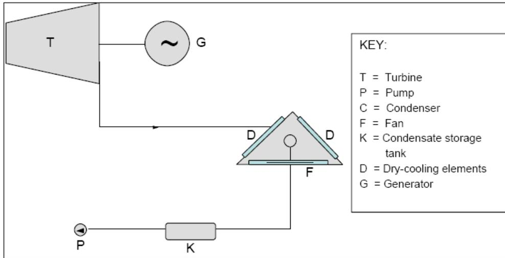
**Figure 2.4** Showing a direct dry cooling system
