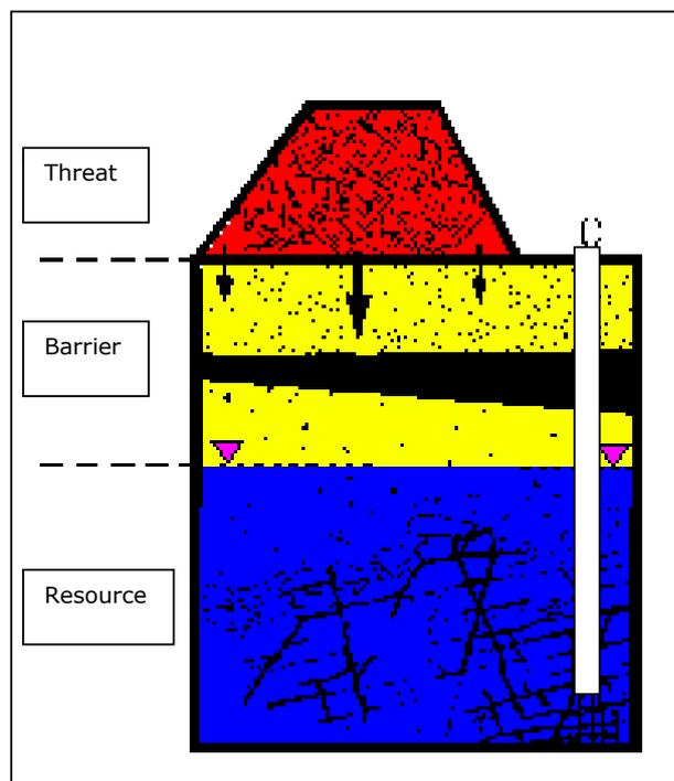
**Figure 6.13:** The assessment criteria to determine site suitability from a groundwater perspective.
