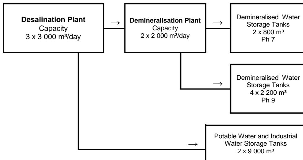
**Figure 3-9: Schematic depiction of the desalination and demineralisation plants**
