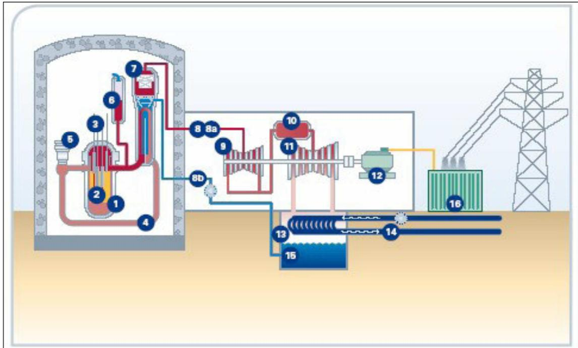
**Figure 3-1: Key features of a Pressurised Water Reactor**
