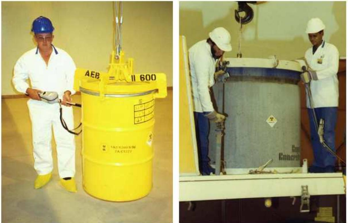
**Figure 3-13: Standard steel and concrete containers used for radioactive waste disposal at Vaalputs**
