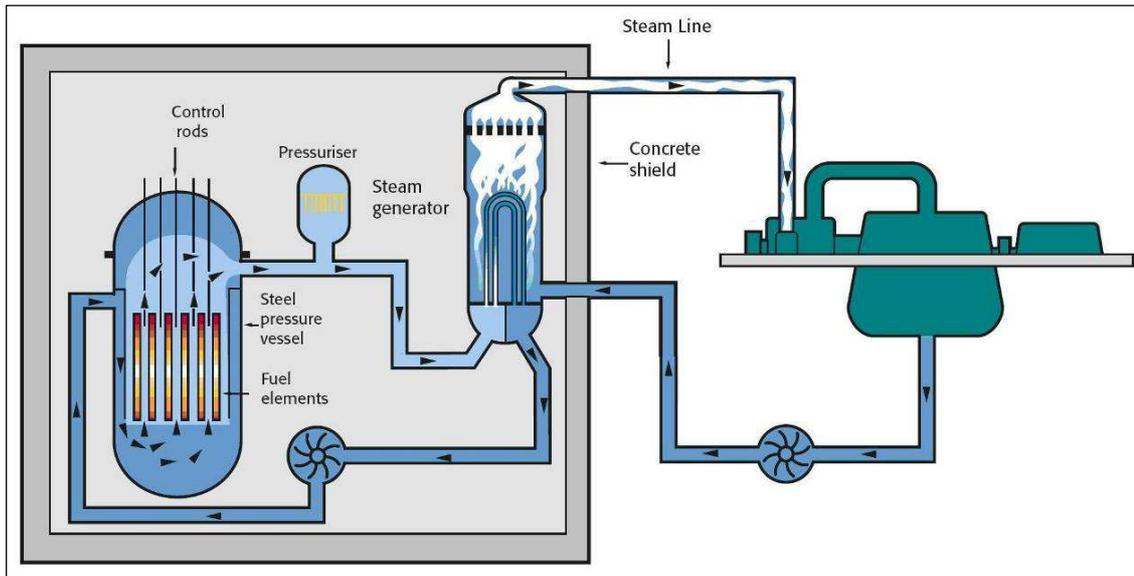
**Figure 3-2: Simplified diagrammatic depiction of a Pressurised Water Reactor (PWR)<sup>6</sup> (Ragheb, 2008)**
