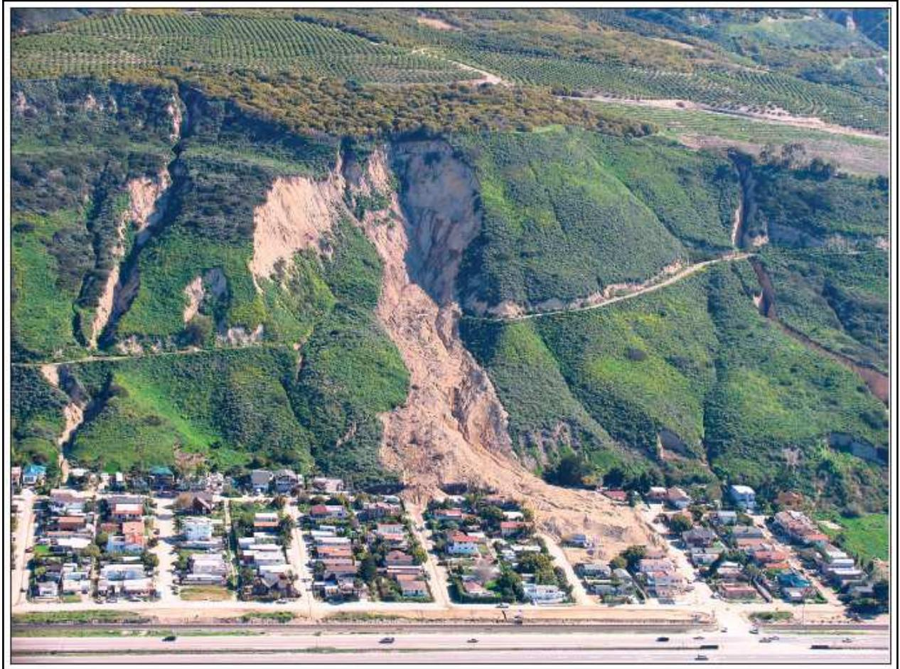
Figure 2.6. Damage caused by a landslide in California. This landslide falls in the debris flow category. From USGS (2010).
