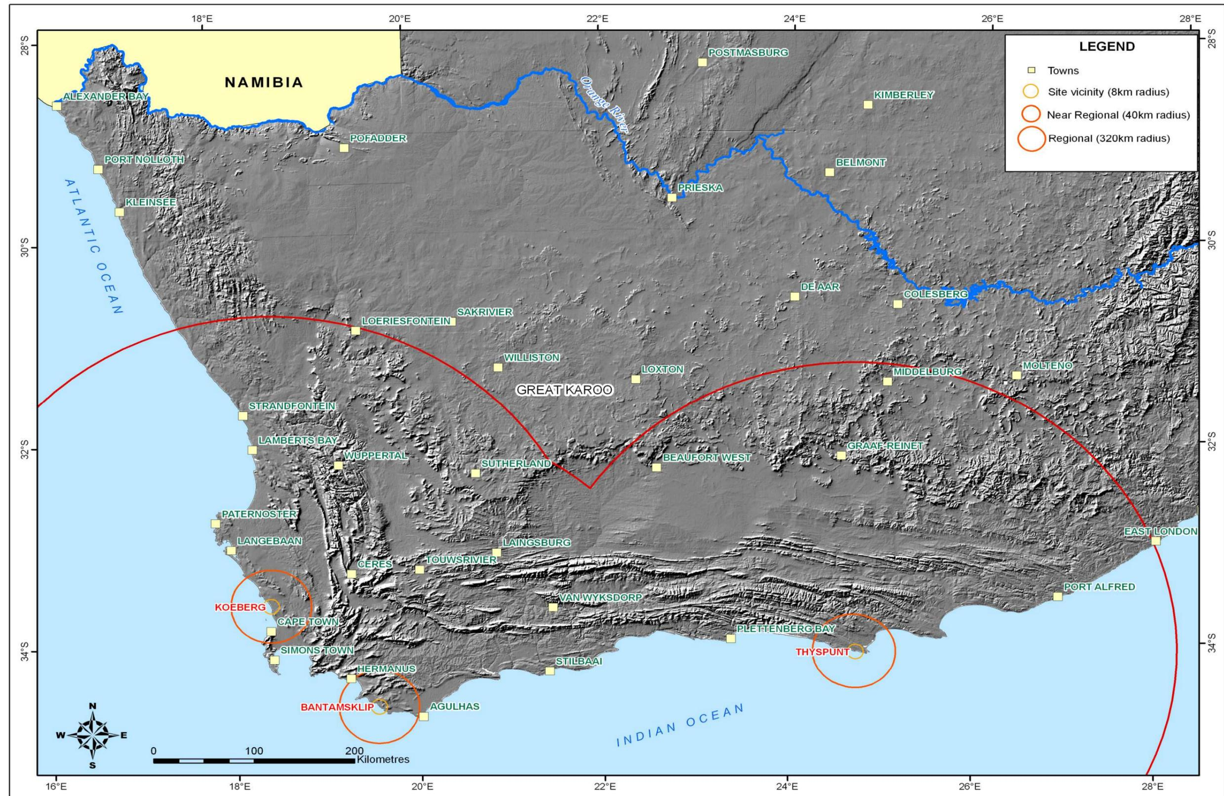
Figure 1.2: Topographic map of the Dufnefontein Site area with the 8 km and 40 km radii that guide geological investigation
