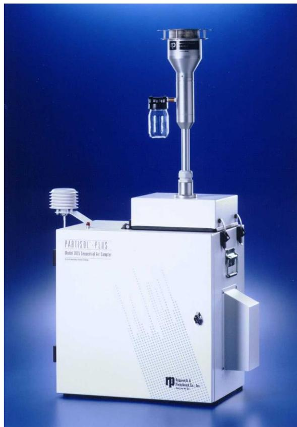
Figure 8-4: Partisol-Plus sequential air sampler.
