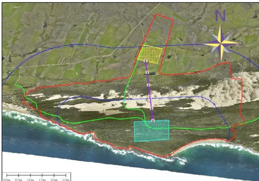
Figure 23: Recommended location for NPS (turquoise diagonal cross-hatching) and HV yard (yellow vertical cross-hatching) on the Thyspunt site (red outline). Recommended route for the 132kV power line is also indicated. 800 m and 3000 m lines from EIA are shown in blue.
