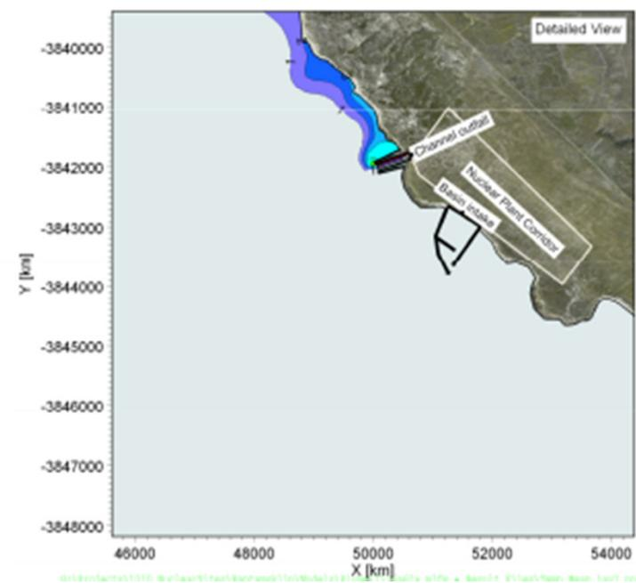
Title: Thermal plume modeling: Mean increase in temperature due to power station at Bantamsklip (Option 2)
