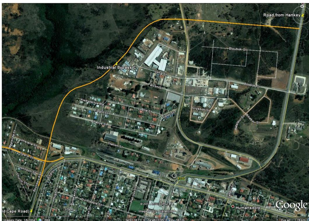
It is proposed that the main entrance into Kruisfontein be moved to Searle Street. Cape Road would be re-aligned to meet with the Industrial Bypass at a crossroad intersection at the end of Searle Street and this would become a major intersection. This would improve the entrance into Kruisfontein which is currently into Johnson Street and is uncontrolled and dangerous for vehicles crossing the Cape Road traffic when entering Kruisfontein from Humansdorp.
