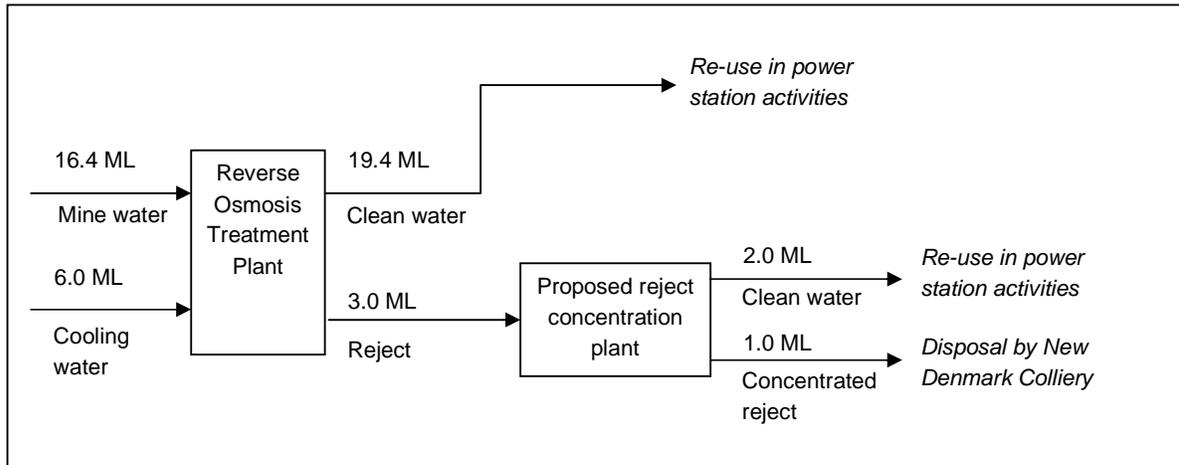
**Figure 3.2 Process flow diagram of daily proposed reject treatment and disposal**
