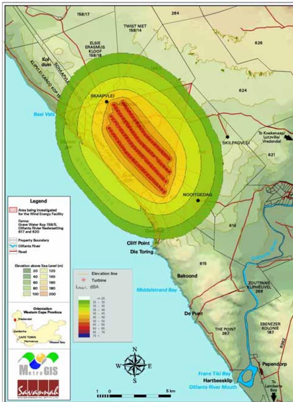
Figure 7.5:  $L_{Req,T}$  contours for 100 wind turbines - maximum sound emission
