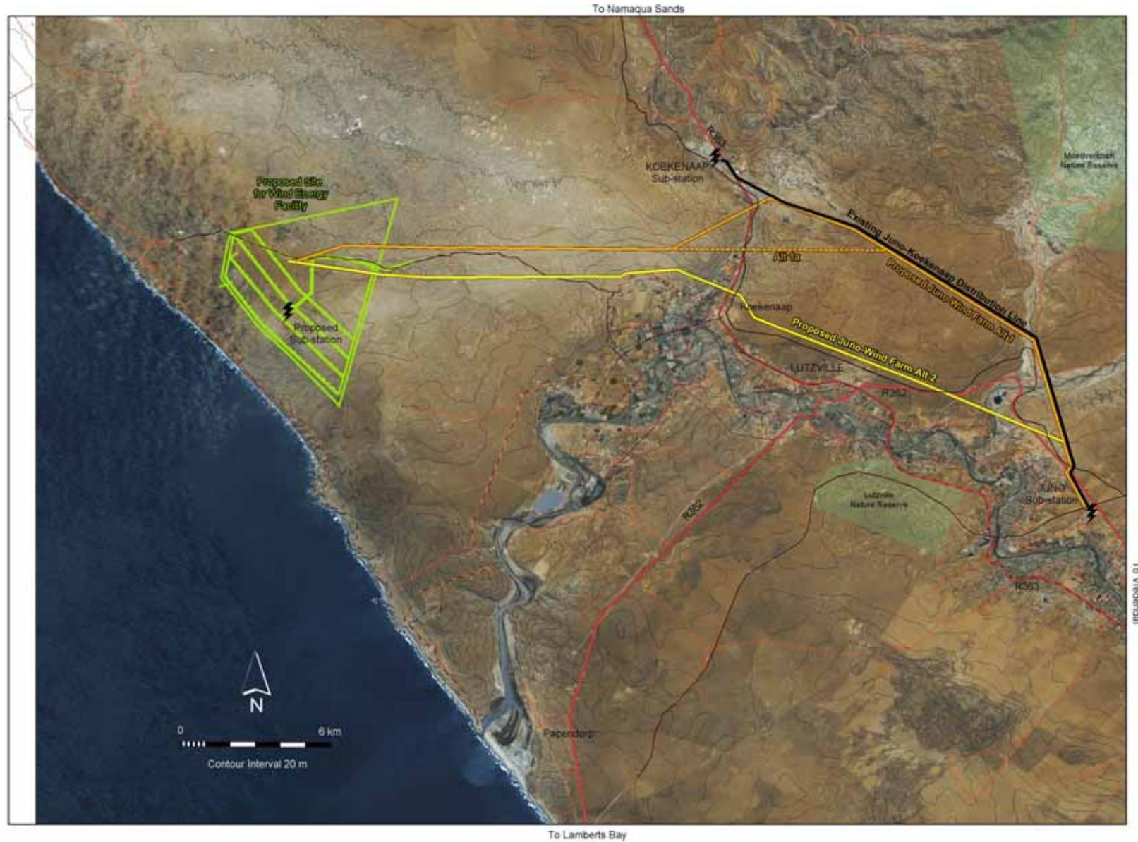
**Figure 9.3:** Alternative power line corridors 1 (and 1a) and 2 identified for consideration in the EIA process
