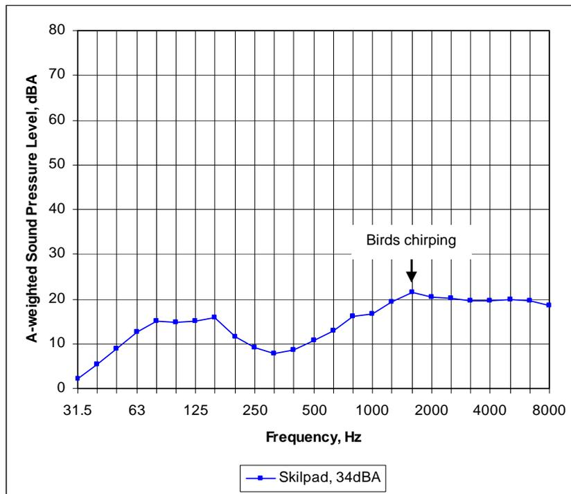
**FIGURE 9 Sound level spectrum measured at location L4 on gravel road to Skaapvlei just beyond turnoff to Skilpadvlei (no photograph)**
