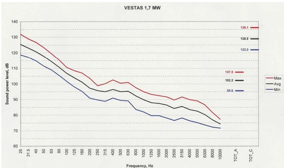
**FIGURE 10 Sound power level emission of a Vestas, V66 wind turbine**
