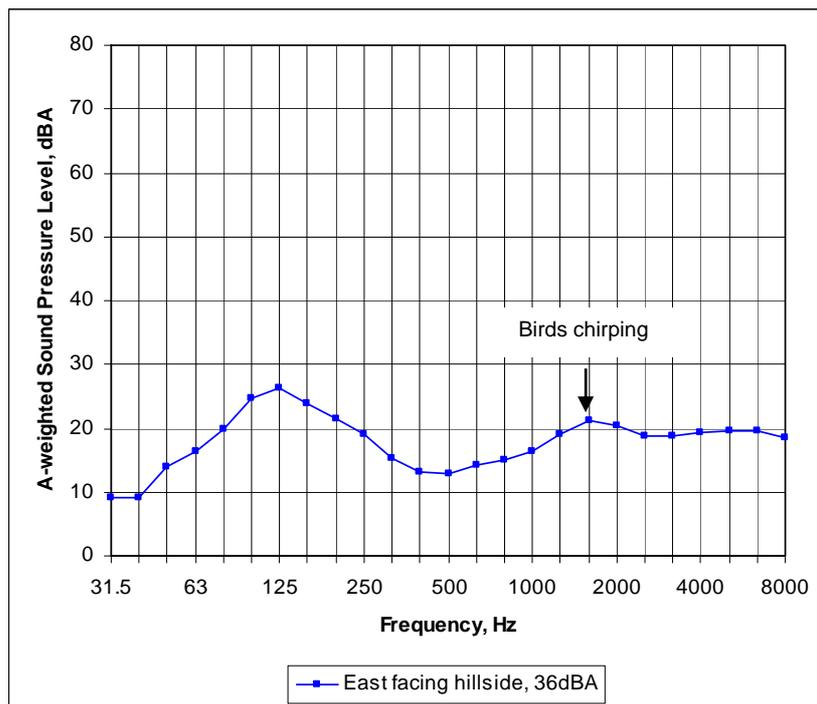
**FIGURE 8 Sound level spectrum measured at location L3**
