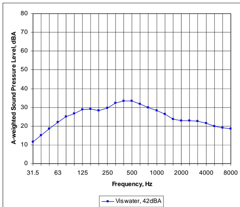
**FIGURE 4** Sound level spectrum measured at L1, Viswater
