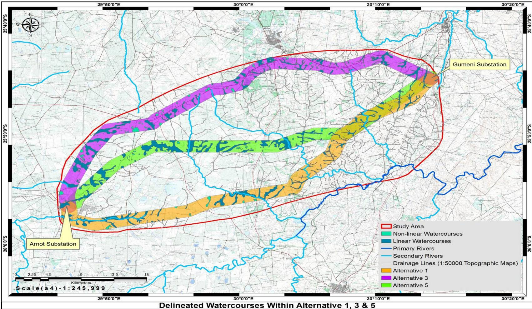
Figure 26: Delineated watercourses based on onscreen digitising within each alternative corridor and watercourses were demarcated as Linear and Non-linear features
