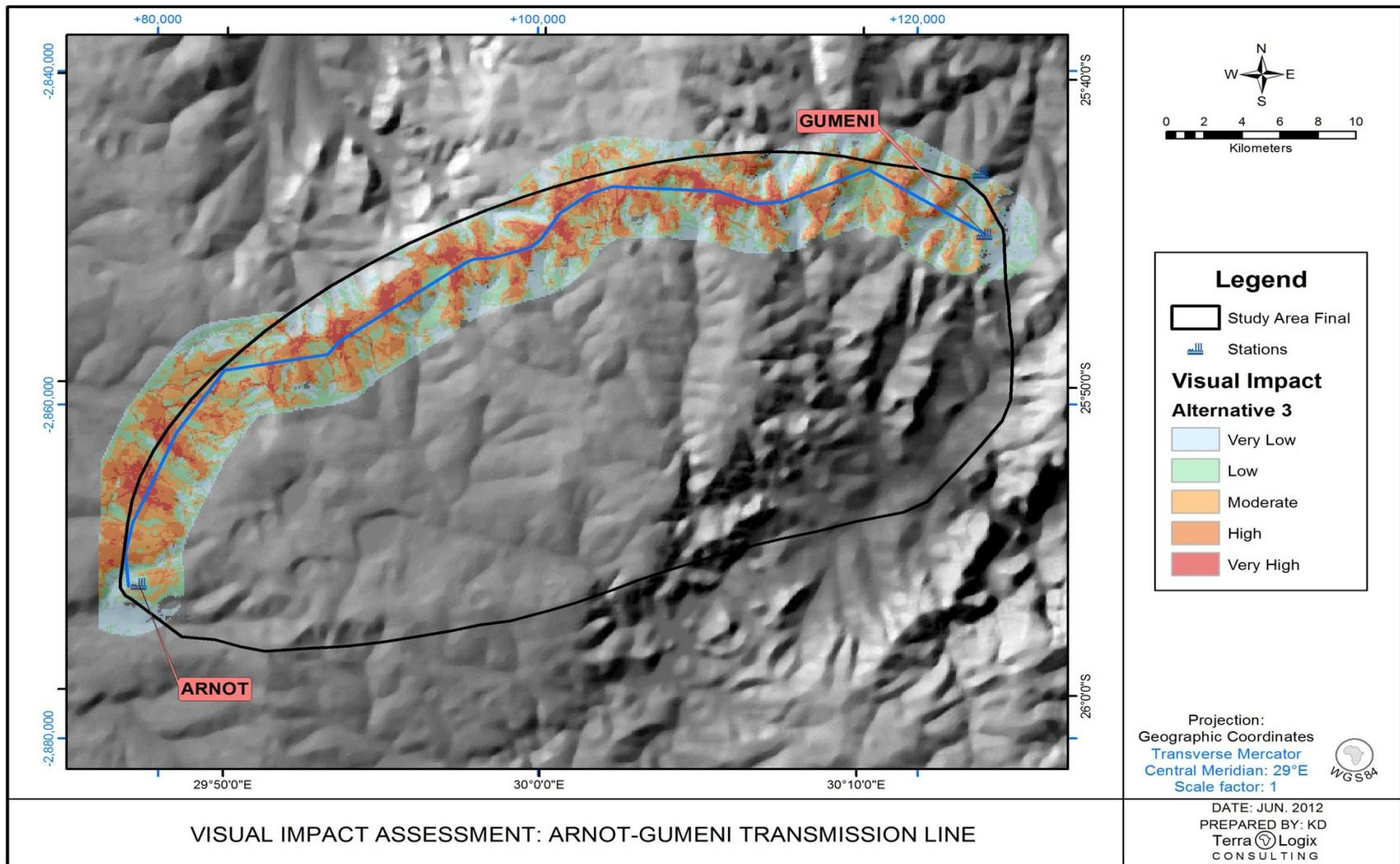
**Figure 33: The results of visual impact on Alternative 3 (Purple corridor) based on model combining the visual sensitivity with the viewshed**
