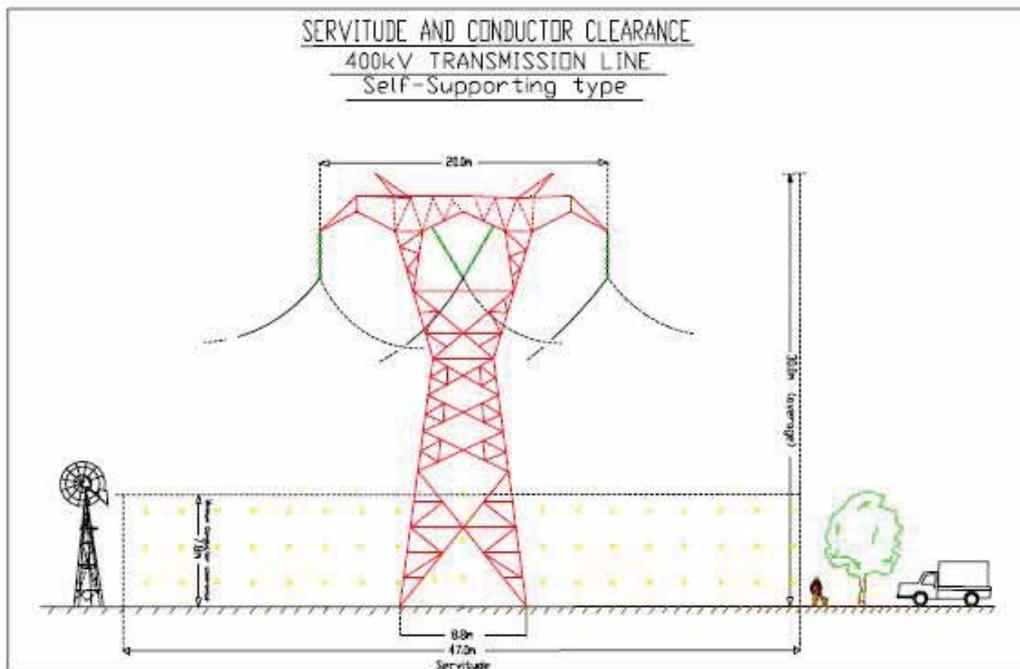
**Figure 2.5:** Diagrammatic representation of the self-supporting strain/bend tower.
