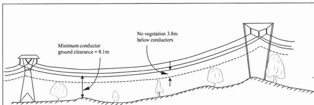
**Figure 2.8:** Servitude requirements in terms of vegetation clearing under conductors and minimum ground clearance
