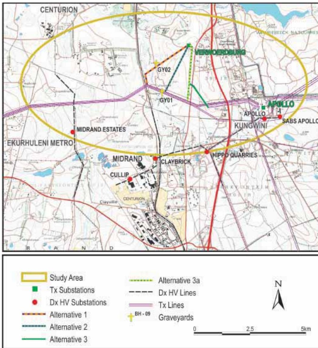
**Figure 3-** Two graveyards located in close proximity to Alternative 01 and Alternative 02, two loop-in and loop-out power lines running between the 400kV Apollo-Pluto power line and the Verwoerdburg Substation (above).
