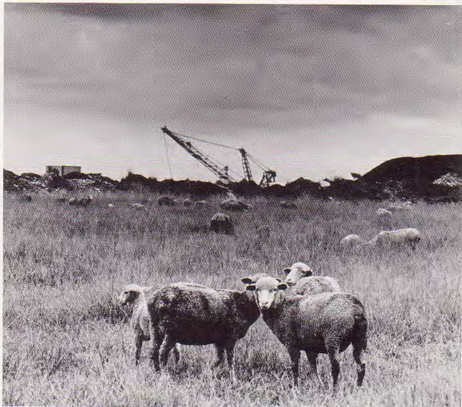
Land disturbed by opencast mining operations to provide coal for Eskom power stations is restored and made available for agricultural use. In this picture, opencast-mining activity is taking place in the background, while the previously disturbed land in the foreground has been restored to pasture.
