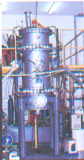
High-temperature steam electrode boiler, an example of electro-technology for end-use customers
