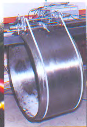
Testing a generator retaining ring for corrosion cracking
