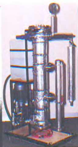
High-temperature steam electrode boiler, an example of electro-technology for end-use customers
