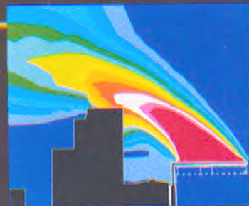
Modelling the air flow around the air-cooled condensers at Matimba
