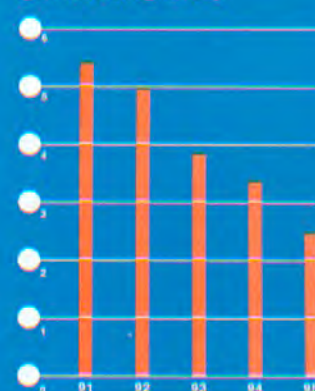
Unplanned automatic grid separations per 7 000 operating hours Coal-fired base-load plant (number per generating unit)
