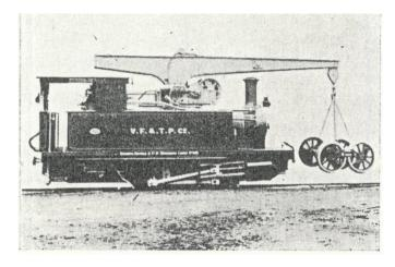
Crane a 3ft 6 in gauge locomotive built in 1913 for the Victoria Falls & Transvaal Power Company
