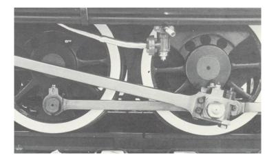
The coup-led wheels of 3 ft 3 in diameter seen here with the water injector in the top centre part of the photograph
