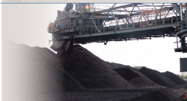
A coal stacker/reclaimer is used for coal handling at the coal stockyard.
