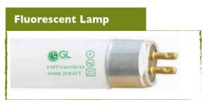
Figure 1 Fluorescent Lamp – F for Fluorescent, 28 for colour code, T5 for diameter, 28 Watt
