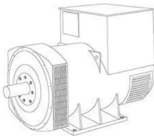
The generator part of the genset will start generating power once the engine starts and will stabilise at around 220 volts until a load or wattage is connected. This is where it is vitally important to decide what load is to be connected to the genset.
