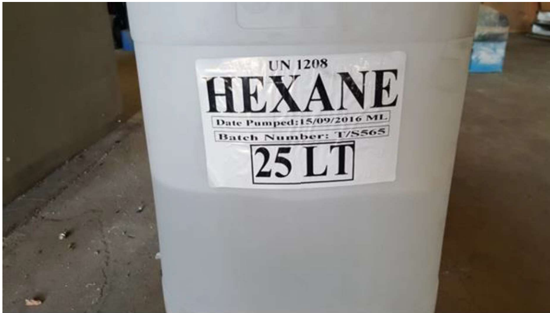
Figure 5. The fuel used in the fire pan is identified by the label on the container from which the fuel was dispensed.
