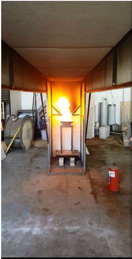
Figure 17: SANS 10177-10 test run and ignition area post-run
