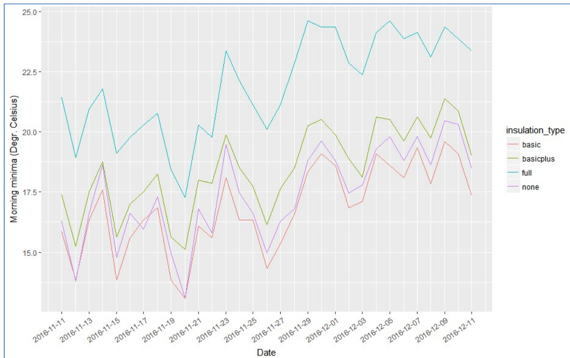
Figure 20 Performance of LPG basic-plus households in terms of instantaneous indoor morning minima, compared to LPG basic, LPG full and control households (Period: 11 Nov - 11 Dec 2016)
