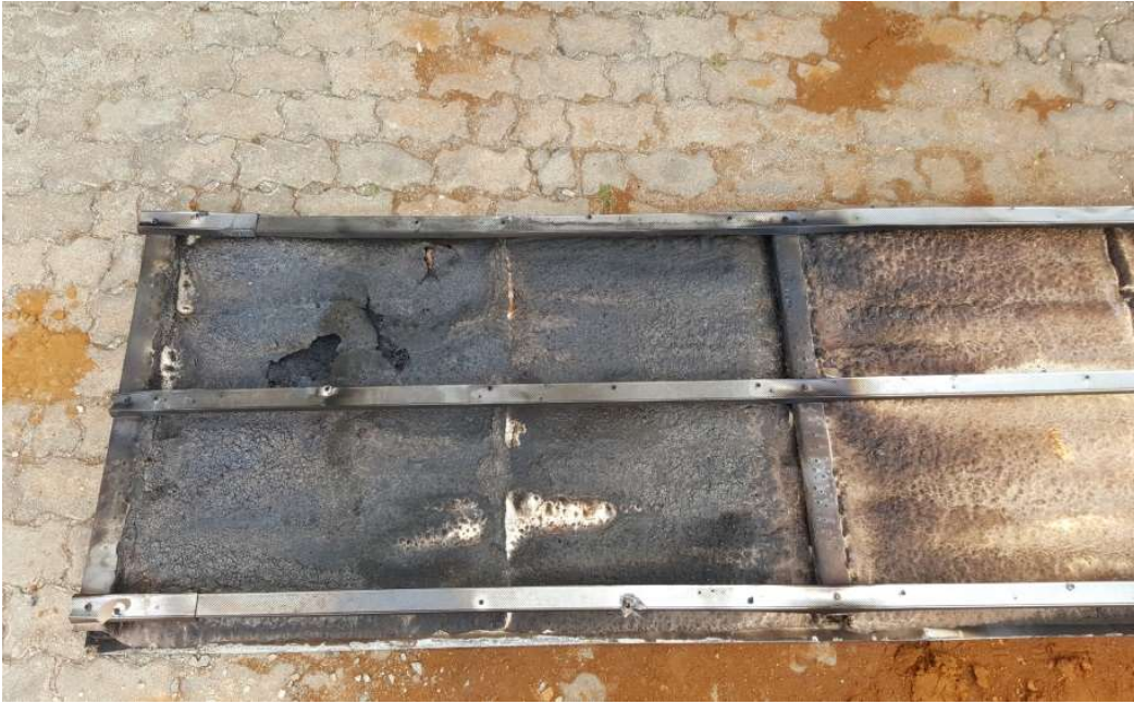
Figure 18: SPF surface in ignition area (<2m)
