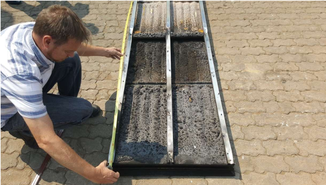
Figure 19: Fire spread analysis
