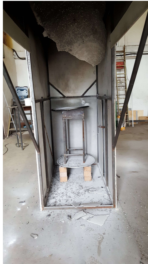
Figure 17: SANS 10177-10 test run and ignition area post-run
