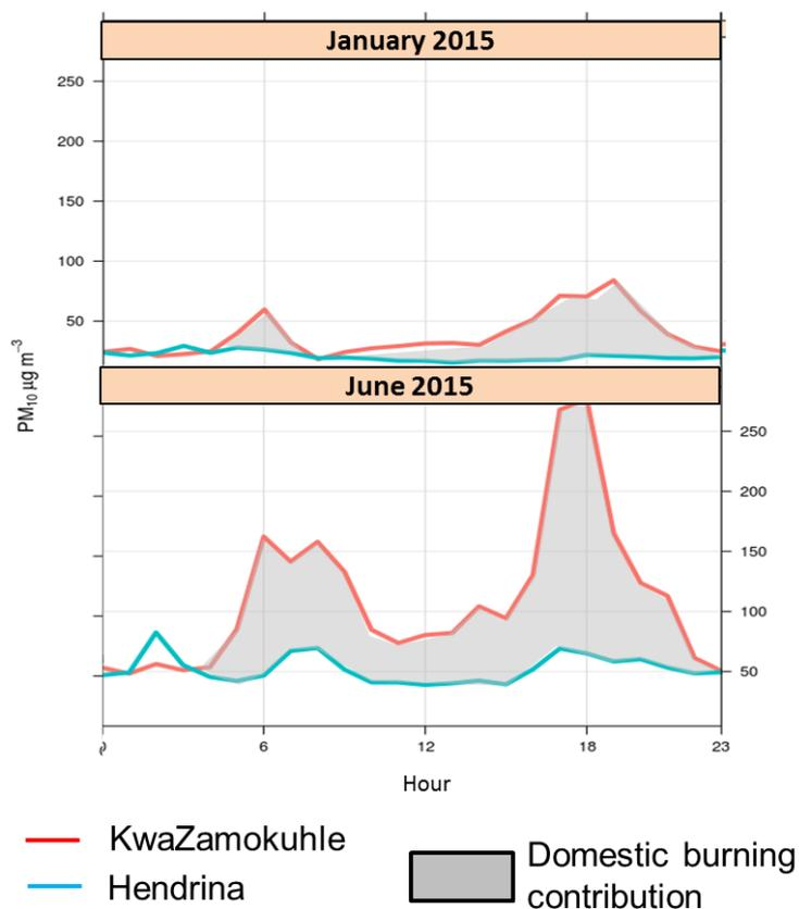
**Figure 6: Average diurnal ambient PM10 concentrations ( $\mu\text{g}/\text{m}^3$ ) measured in KwaZamokuhle and neighbouring Hendrina in summer (January 2015) and winter (June 2015). The difference in concentration between the two areas, shaded in grey, is mainly due to domestic burning in KwaZamokuhle.**
