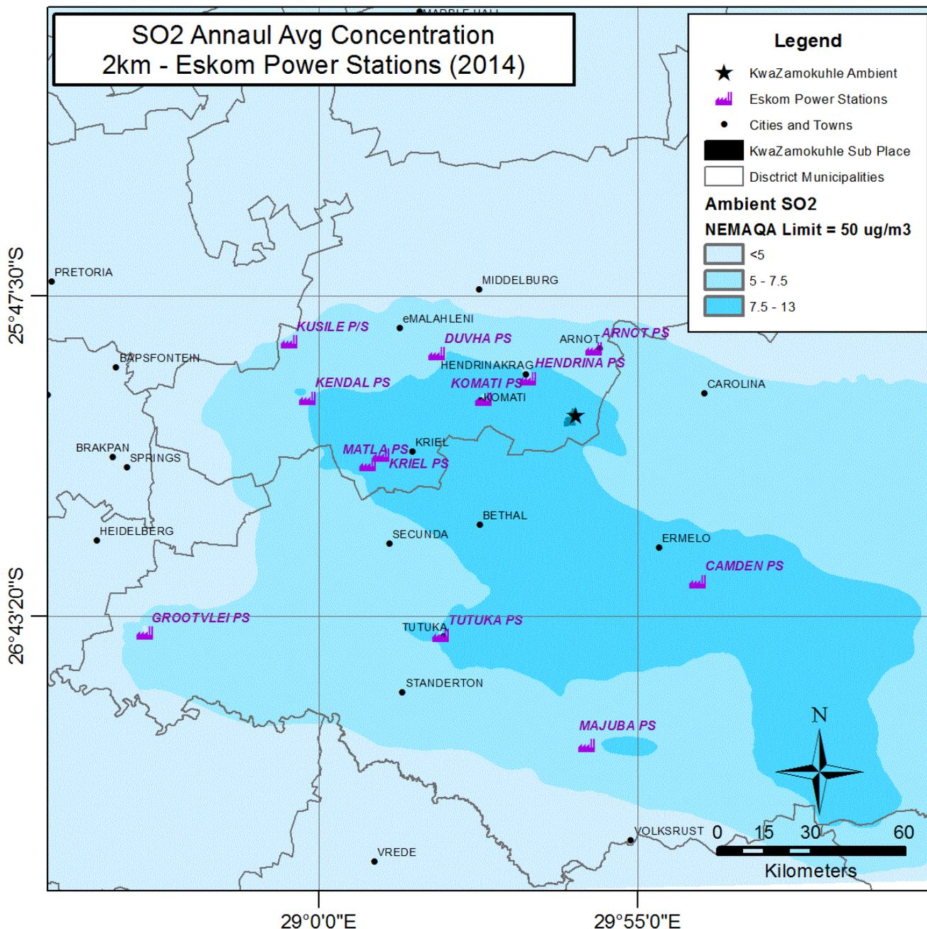
Figure 15: Annual average SO<sub>2</sub> concentrations (µg/m<sup>3</sup>) resulting from SO<sub>2</sub> emissions from all Eskom’s coal-fired power stations in Mpumalanga.
