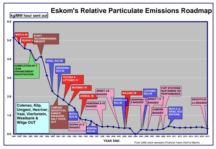
Figure 2: Change in relative emissions of particulates (ash) from Eskom's power stations from the early 1980s to present. Upgrades on power stations to reduce emissions are indicated ('bagged' refers to fabric filter plant retrofits;  $(SO_3)$ ' refers to the installation of SO<sub>3</sub> plants which improve the efficiency of the electrostatic precipitators). Newer power stations have more efficient abatement technology
