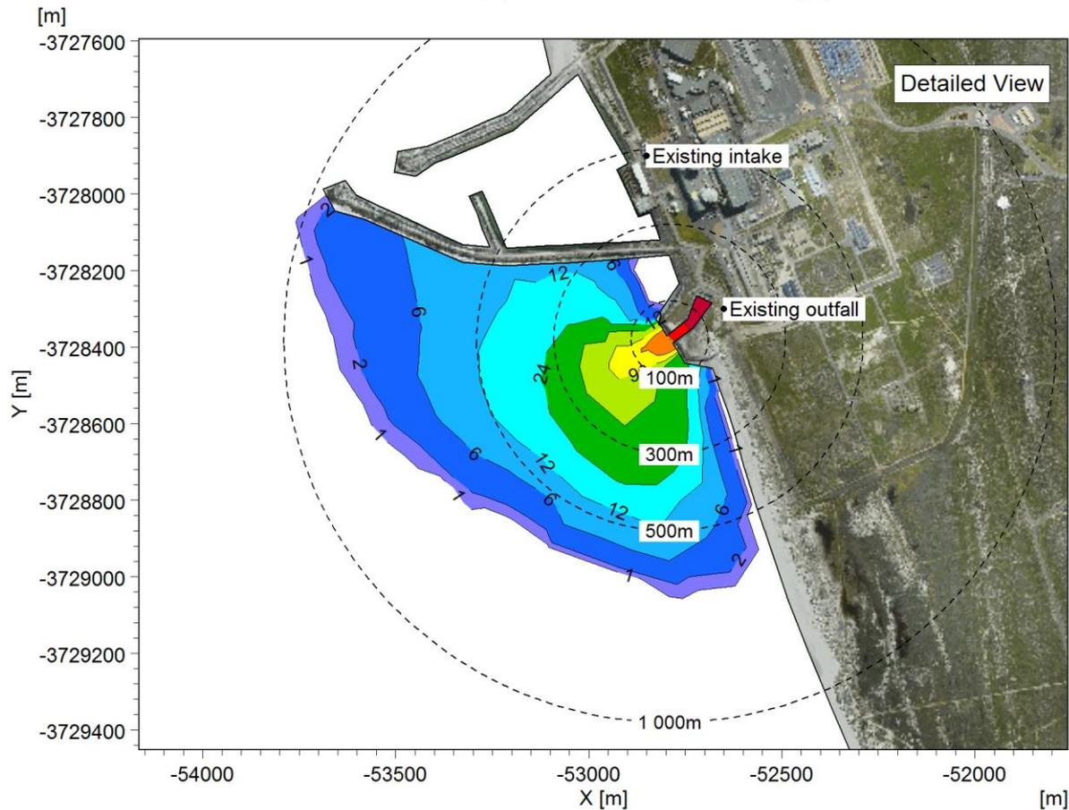
**Figure A-19: Duration that the chronic threshold of 25°C is exceeded near the surface: Case 3 (one unit operational, 60% power).**
