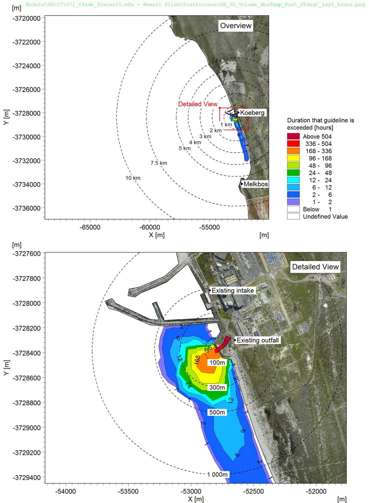
**Figure A-26: Duration that the chronic threshold of 25°C is exceeded near the seabed: Case 6 (two units operational, 100% power).**
