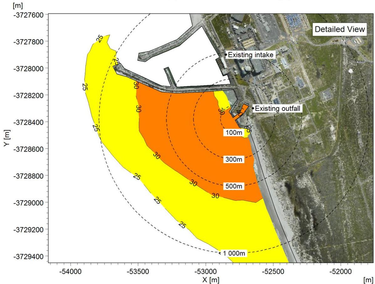
Figure 4-2: Maximum absolute temperature near the surface: Case 1 (one unit operational, 100% power).
