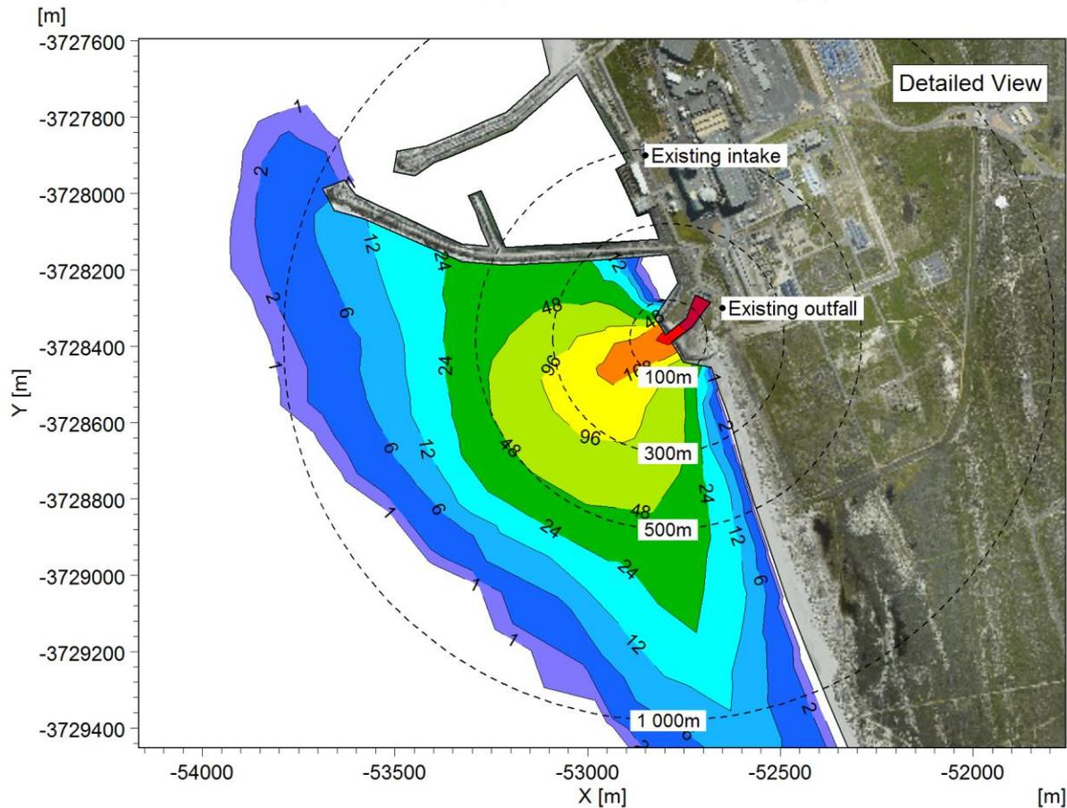
Figure A-15: Duration that the chronic threshold of 25°C is exceeded near the surface: Case 1 (one unit operational, 100% power).
