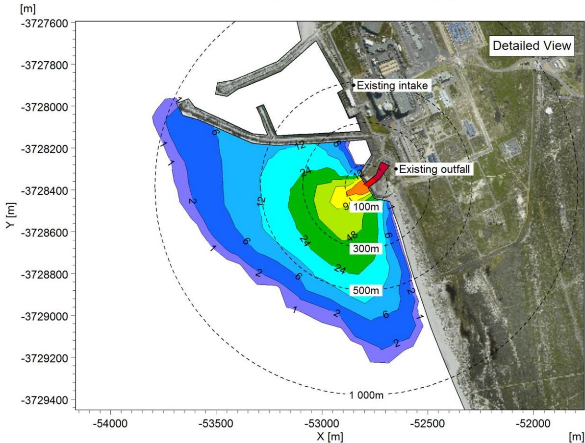
Figure A-17: Duration that the chronic threshold of 25°C is exceeded near the surface: Case 2 (one unit operational, 70% power).
