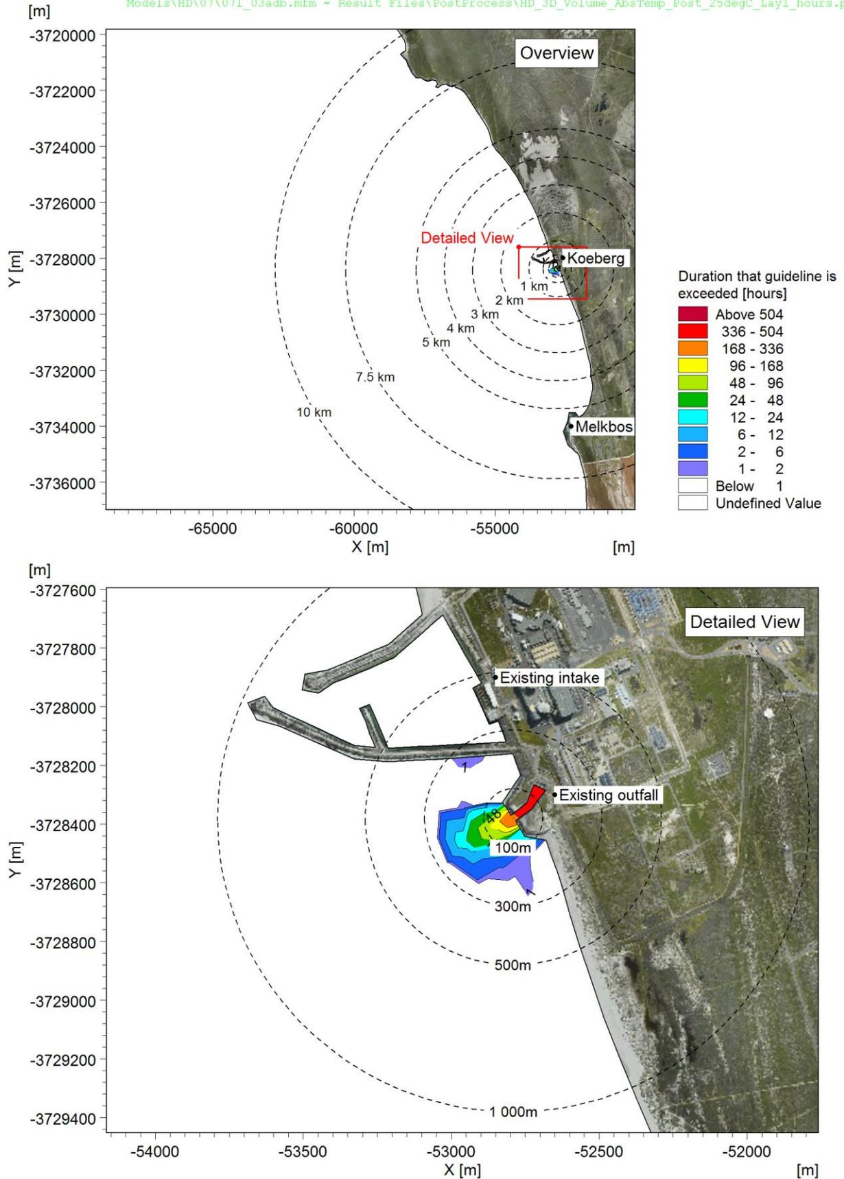
**Figure A-24: Duration that the chronic threshold of 25°C is exceeded near the seabed: Case 5 (one unit operational, 40% power).**
