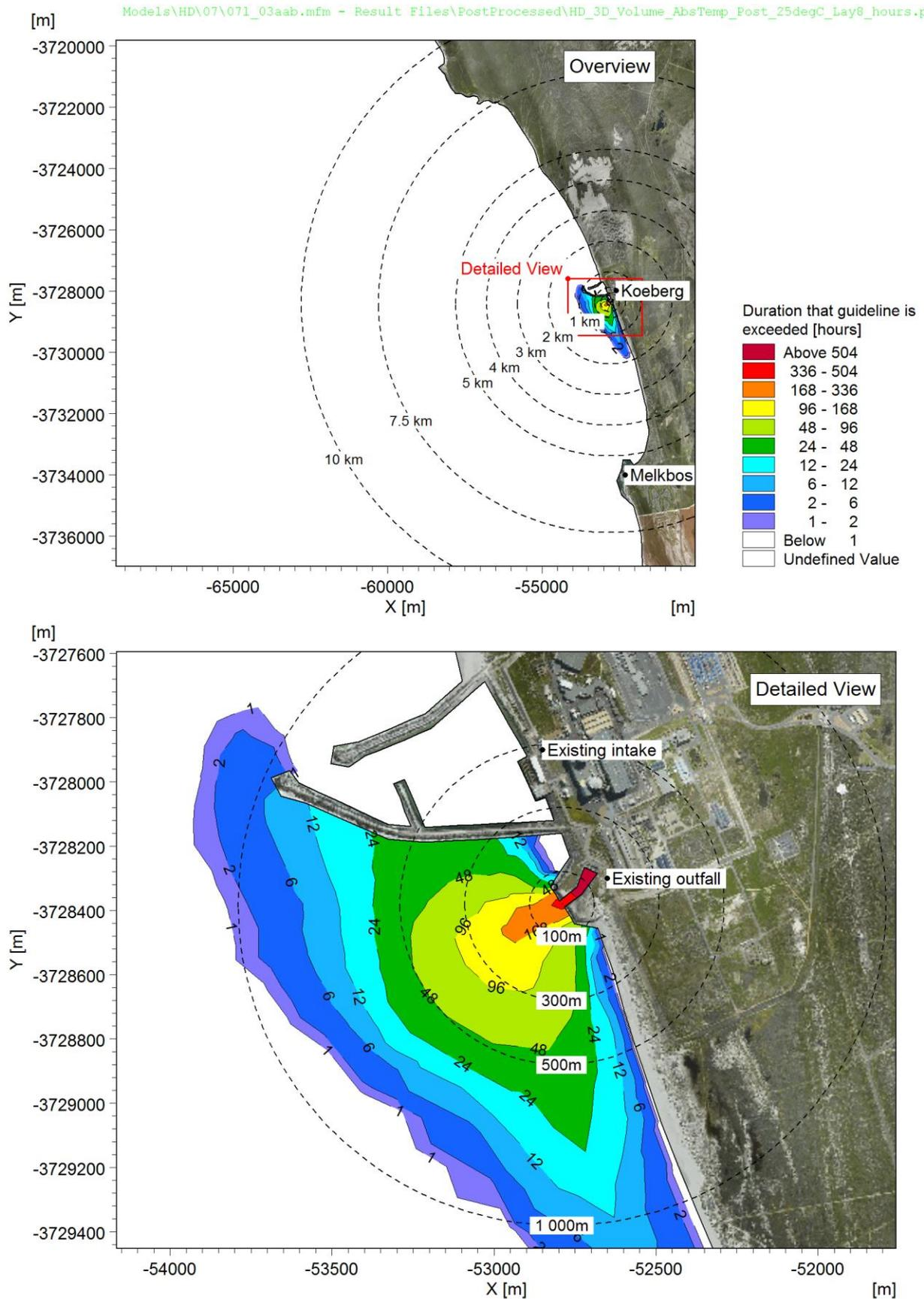
**Figure 4-4: Duration that the chronic threshold of 25°C is exceeded near the surface: Case 1 (one unit operational, 100% power).**
