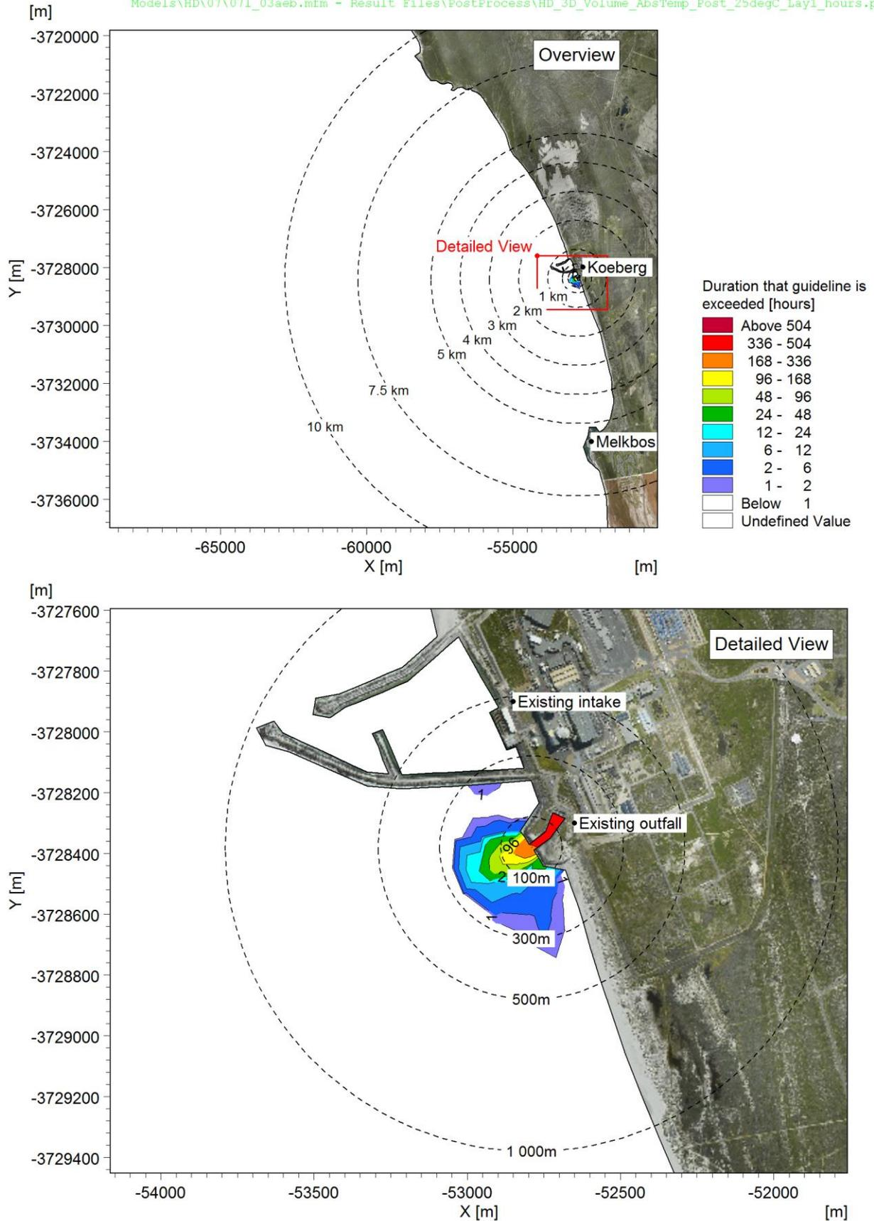
**Figure A-20: Duration that the chronic threshold of 25°C is exceeded near the seabed: Case 3 (one unit operational, 60% power).**
