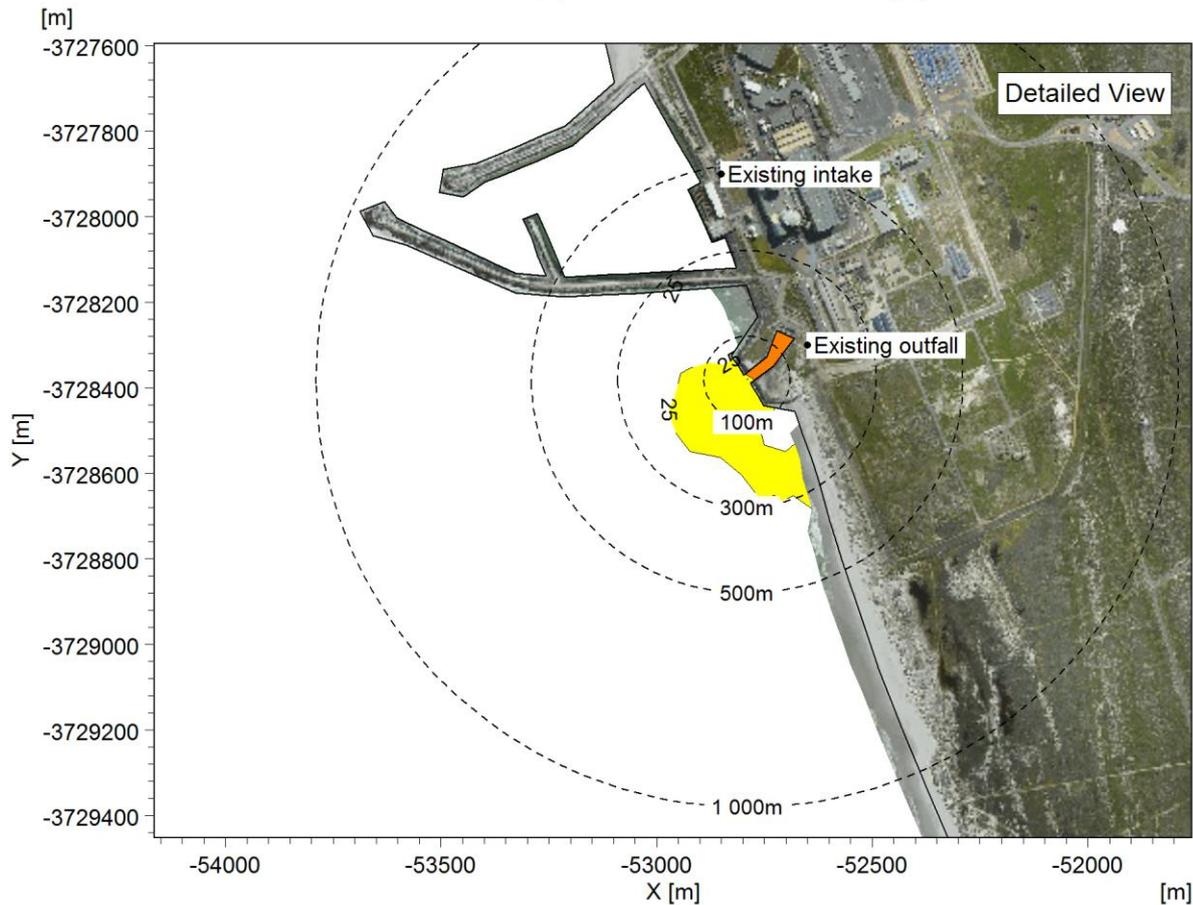
Figure A-10: Maximum absolute temperature near the seabed: Case 5 (one unit operational, 40% power).
