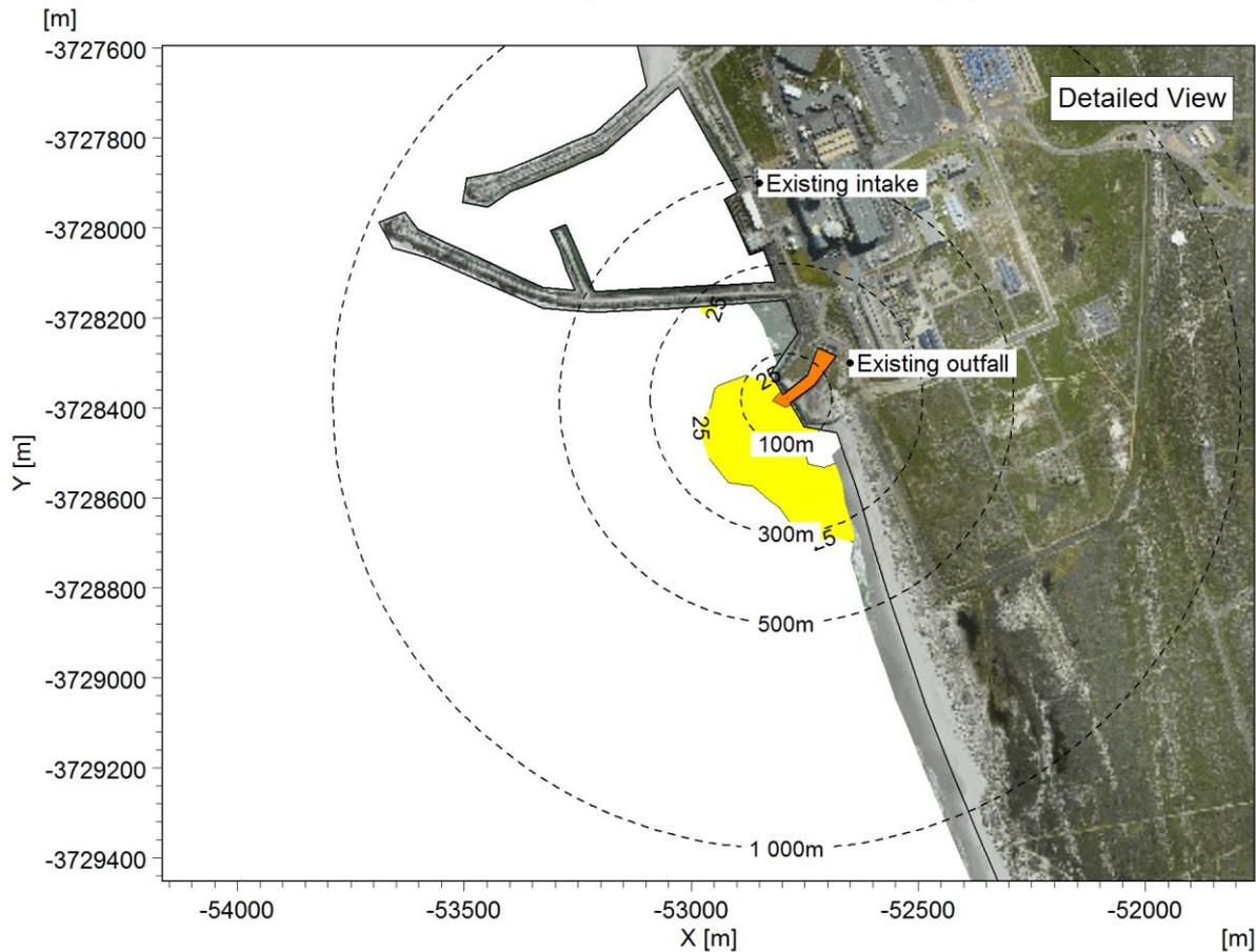
Figure A-8: Maximum absolute temperature near the seabed: Case 4 (one unit operational, 50% power).
