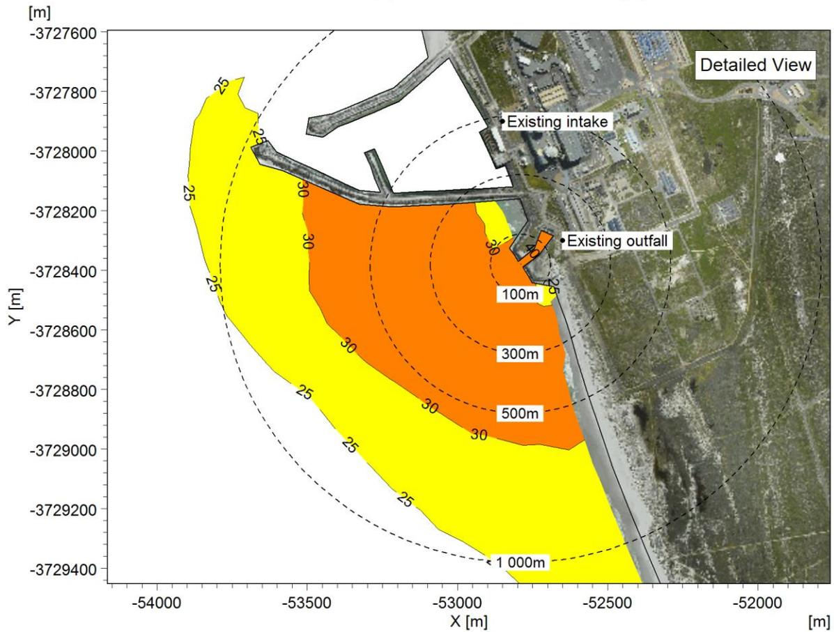
Figure A-1: Maximum absolute temperature near the surface: Case 1 (one unit operational, 100% power).
