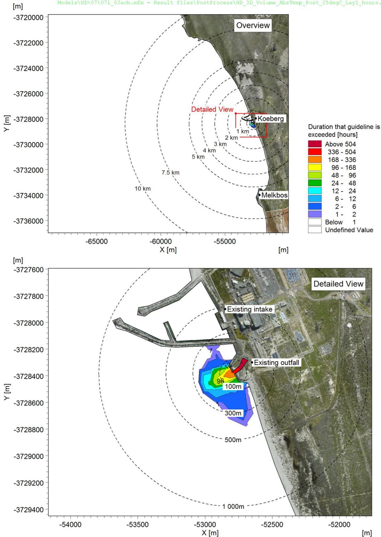
**Figure A-18: Duration that the chronic threshold of 25°C is exceeded near the seabed: Case 2 (one unit operational, 70% power).**
