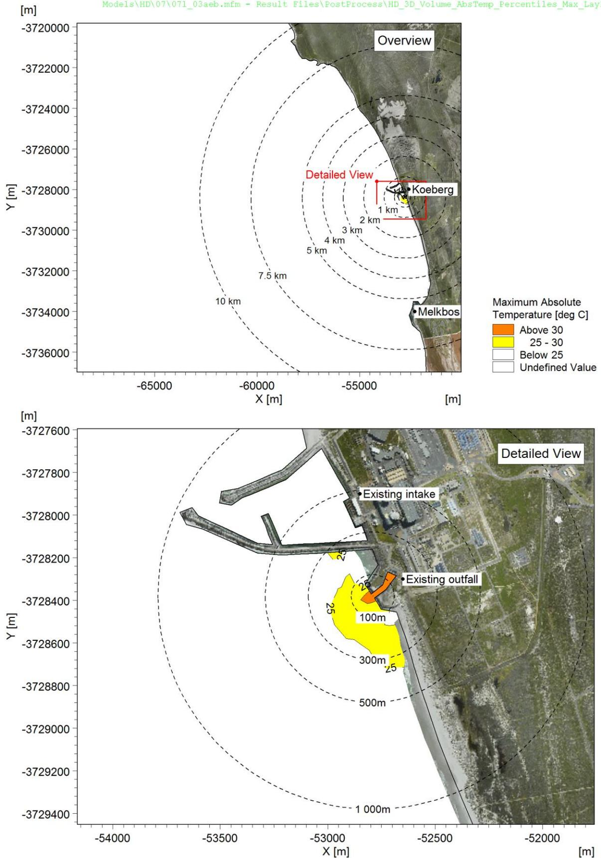
Figure A-6: Maximum absolute temperature near the seabed: Case 3 (one unit operational, 60% power).
