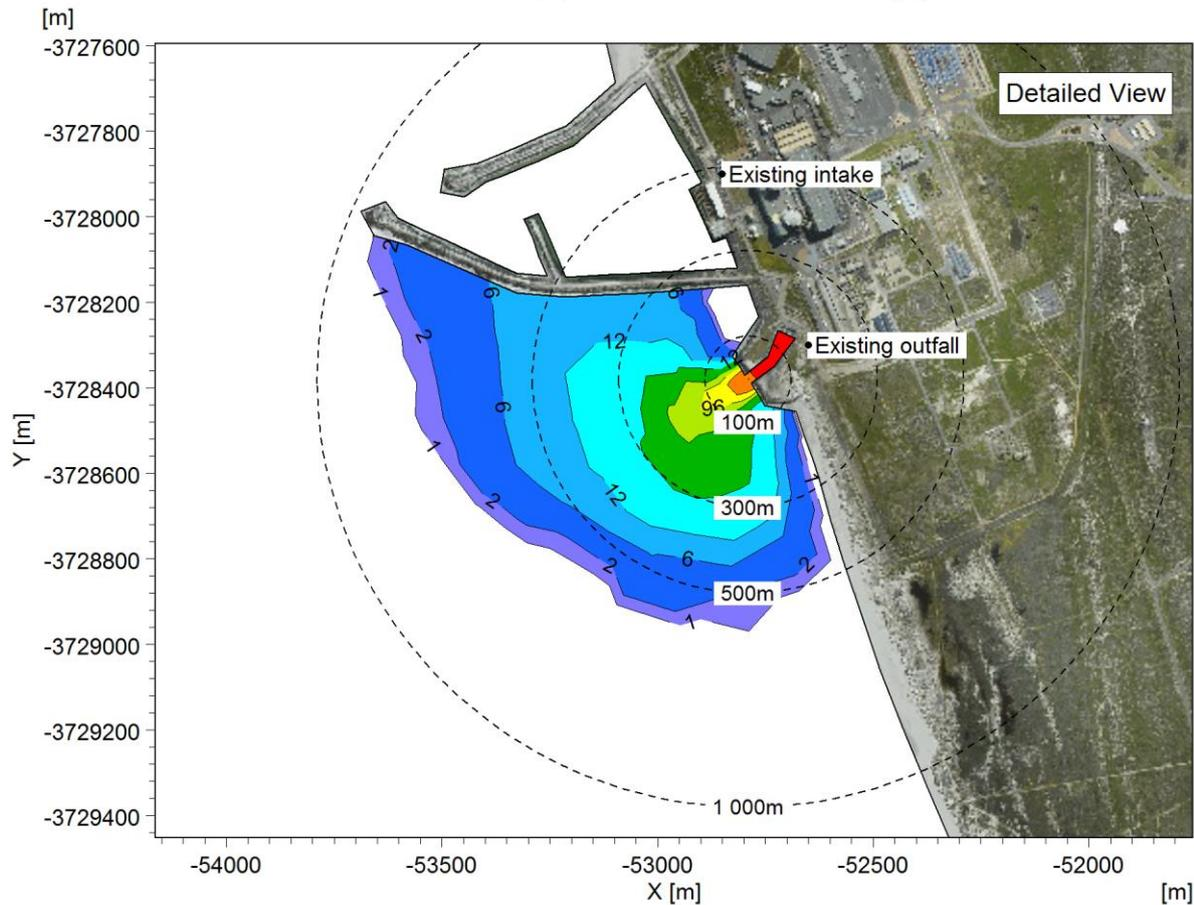
**Figure A-23: Duration that the chronic threshold of 25°C is exceeded near the surface: Case 5 (one unit operational, 40% power).**
