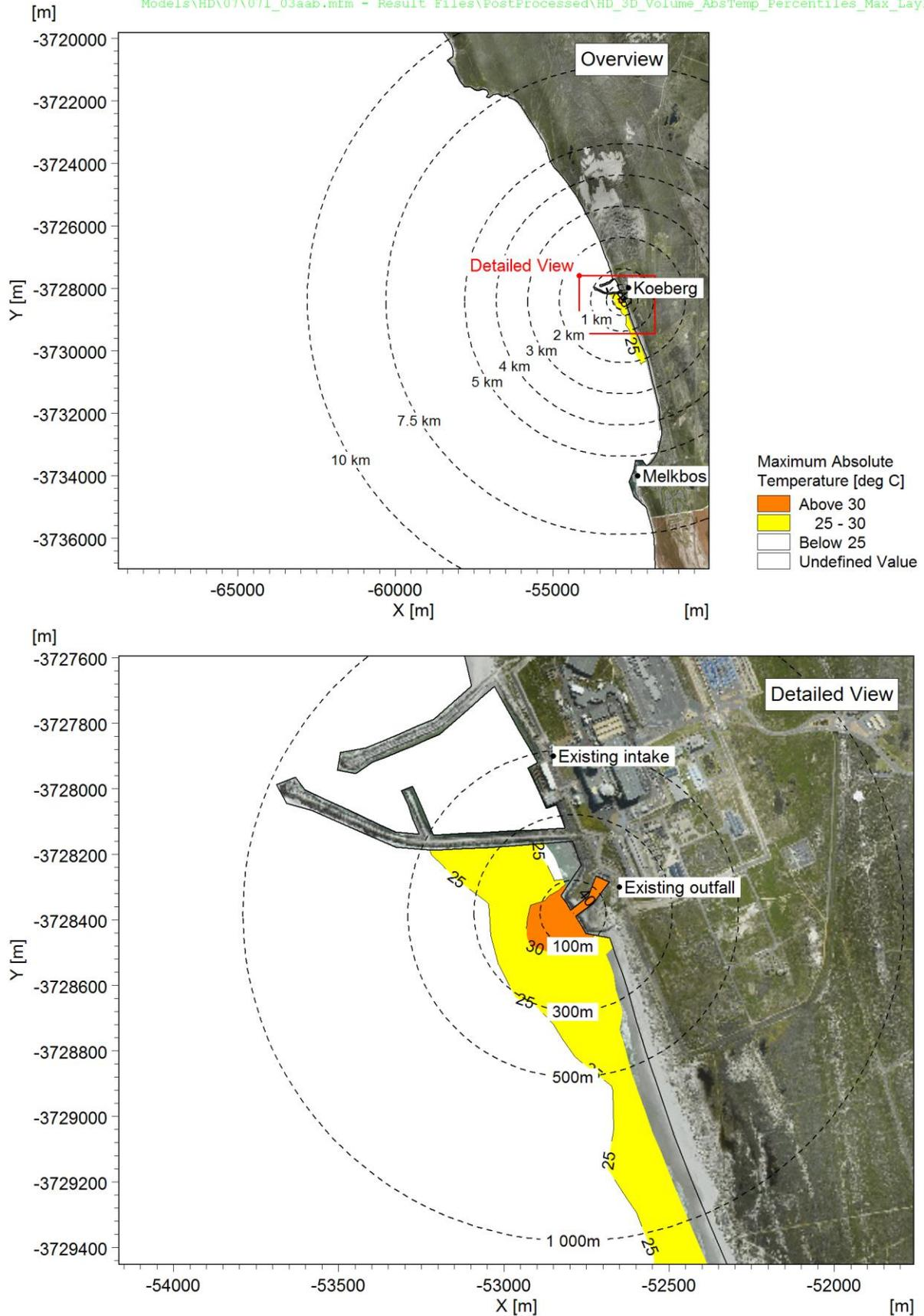
Figure A-2: Maximum absolute temperature near the seabed: Case 1 (one unit operational, 100% power).
