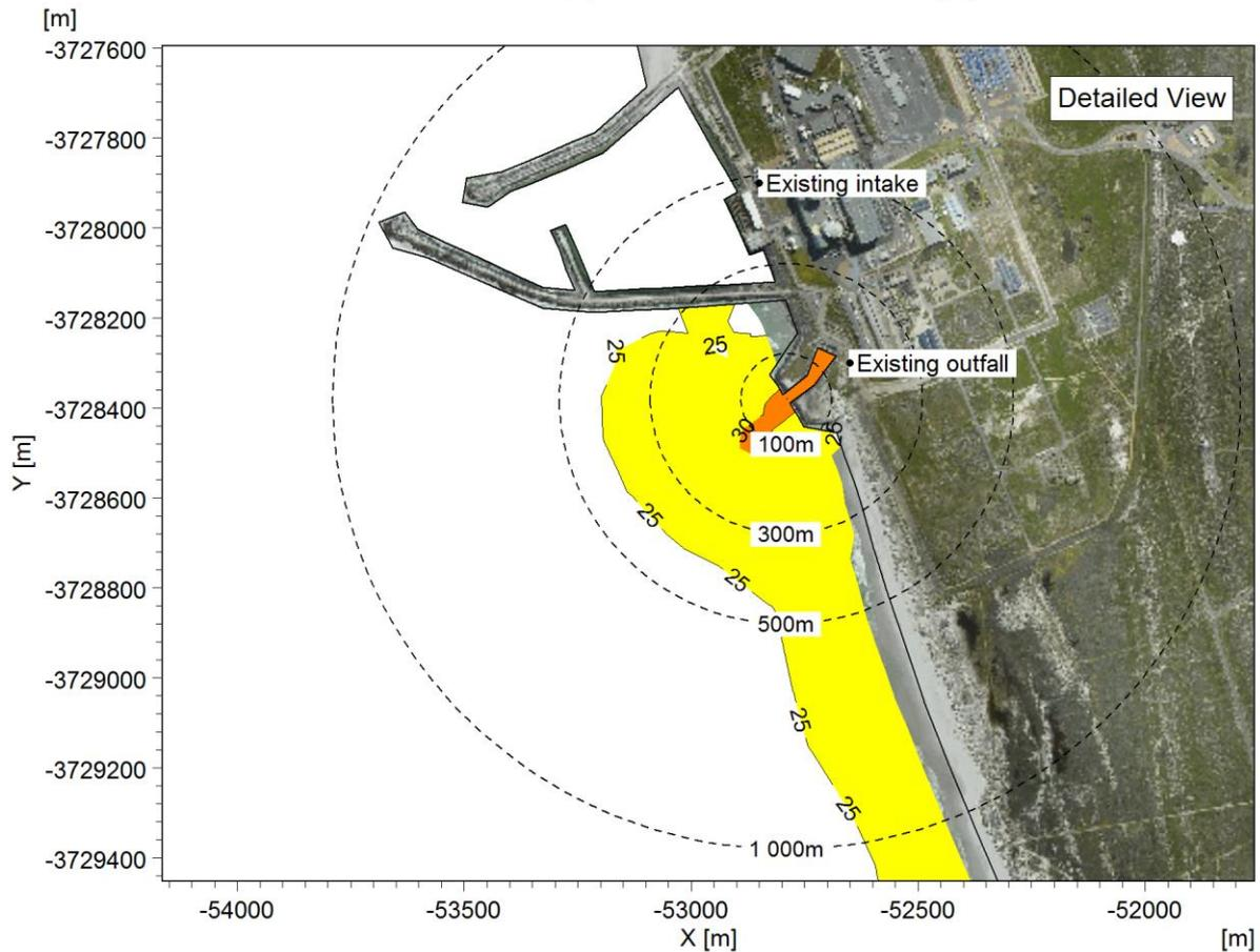
Figure A-14: Maximum absolute temperature near the seabed: Case 7 (two units operational, 70% power).
