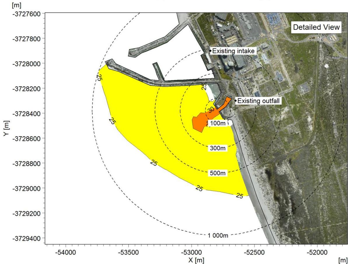
Figure A-5: Maximum absolute temperature near the surface: Case 3 (one unit operational, 60% power).
