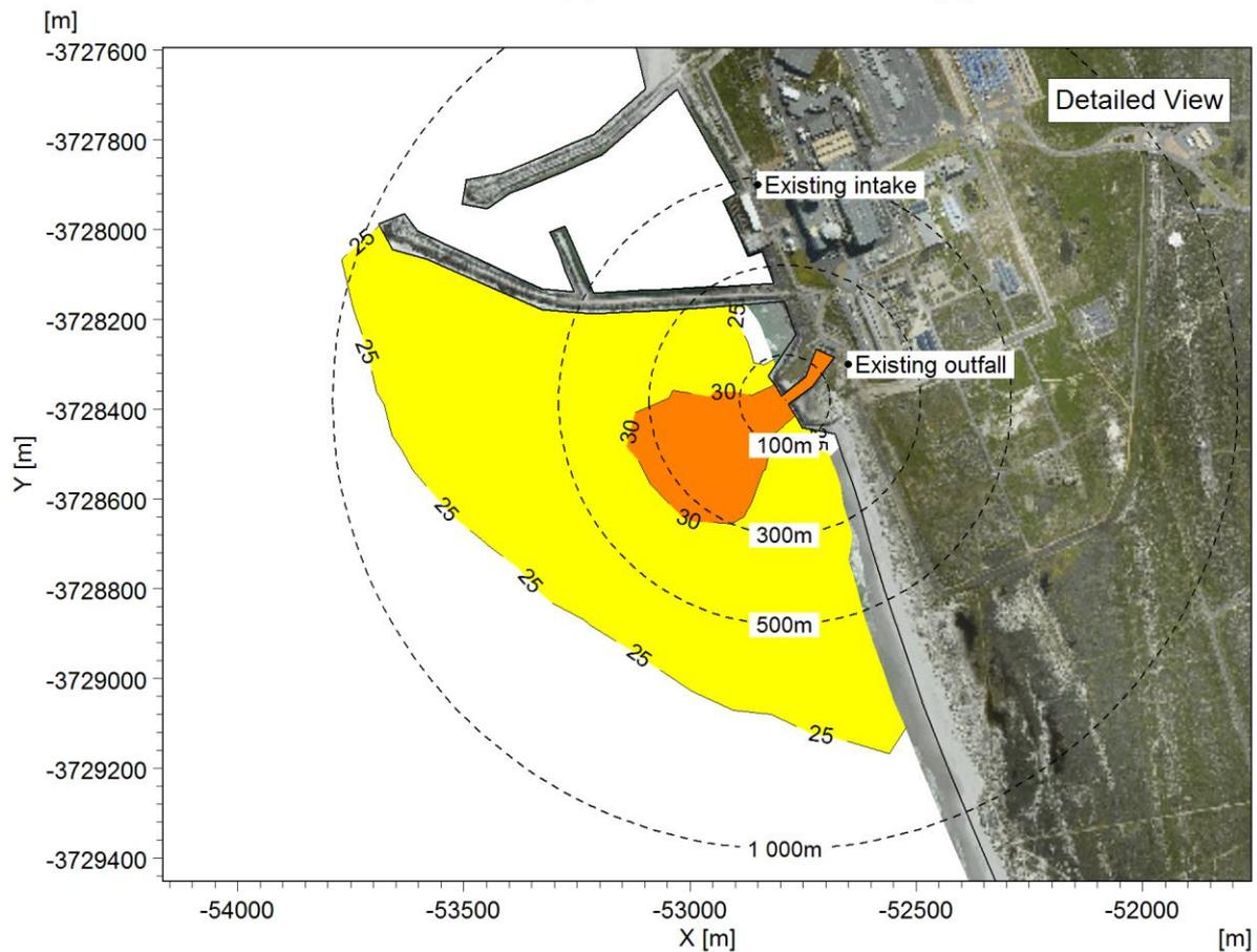
Figure A-3: Maximum absolute temperature near the surface: Case 2 (one unit operational, 70% power).
