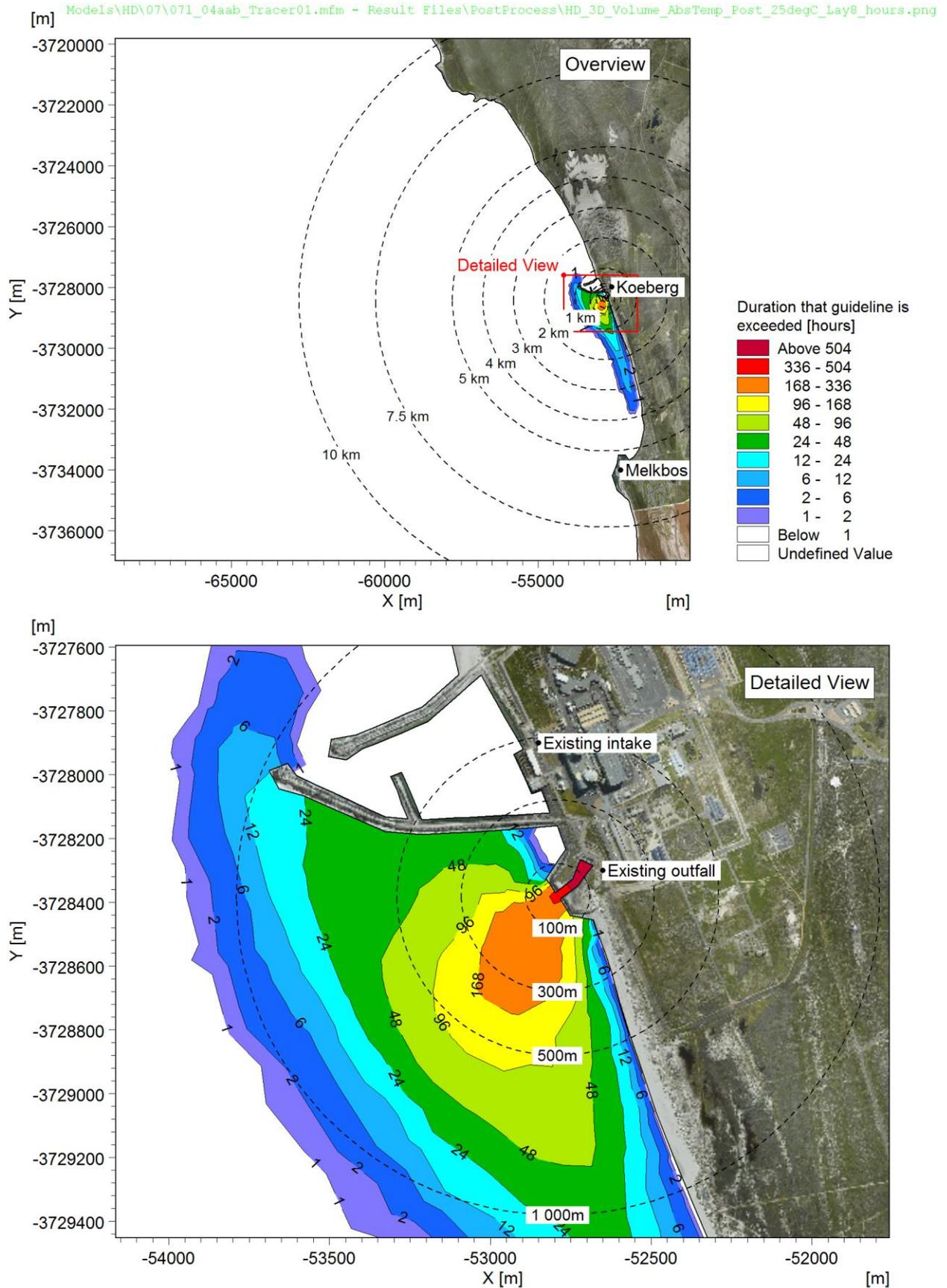
**Figure A-25: Duration that the chronic threshold of 25°C is exceeded near the surface: Case 6 (two units operational, 100% power).**
