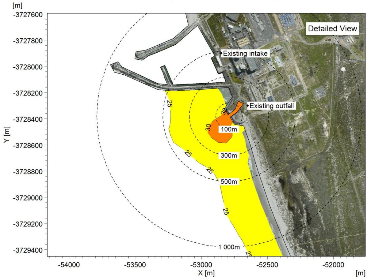
Figure A-12: Maximum absolute temperature near the seabed: Case 6 (two units operational, 100% power).
