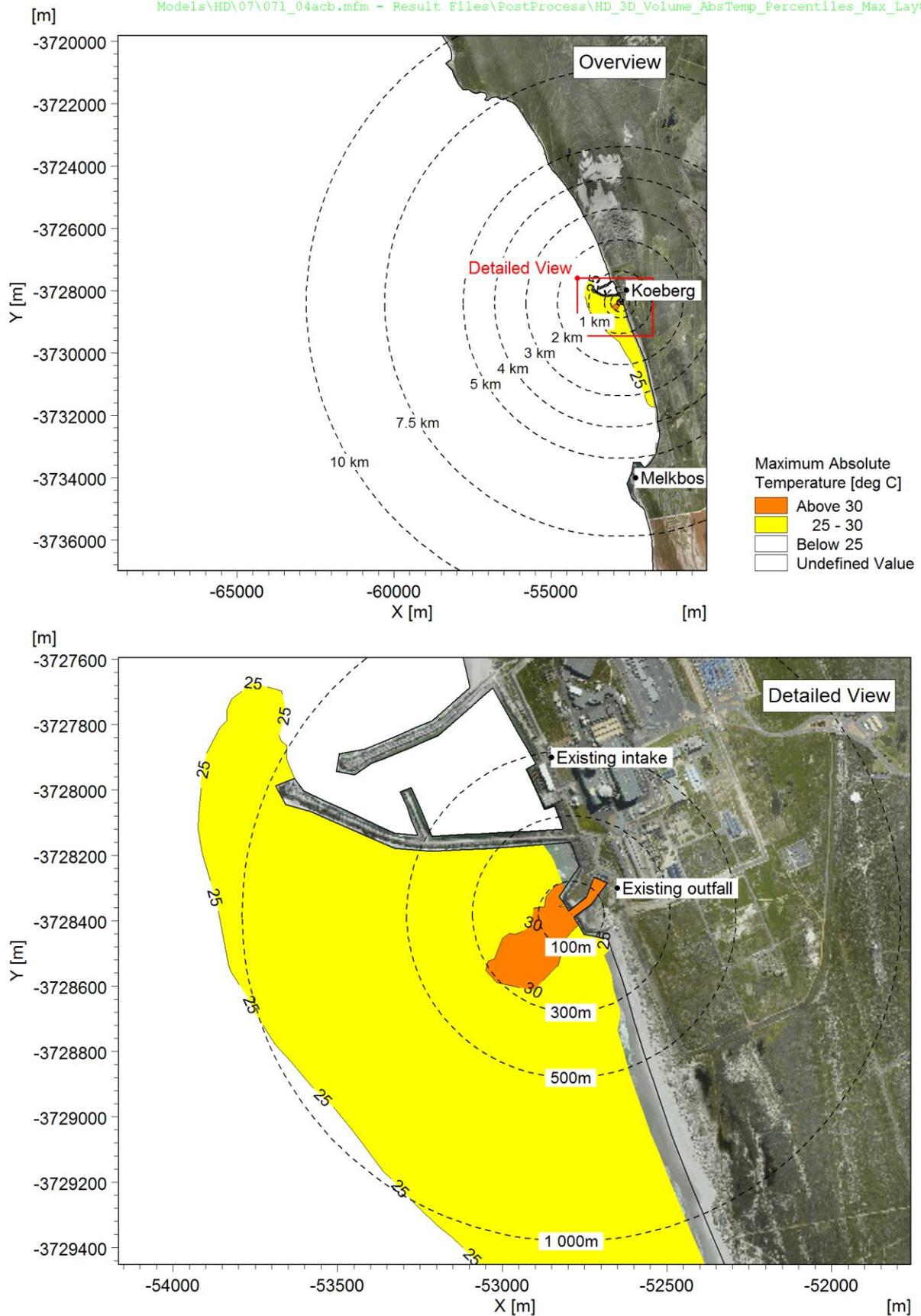
Figure A-13: Maximum absolute temperature near the surface: Case 7 (two units operational, 70% power).
