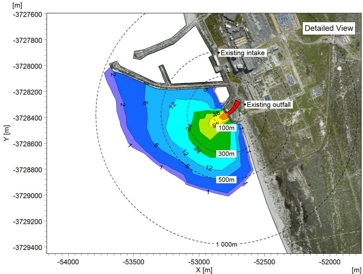
**Figure A-21: Duration that the chronic threshold of 25°C is exceeded near the surface: Case 4 (one unit operational, 50% power).**
