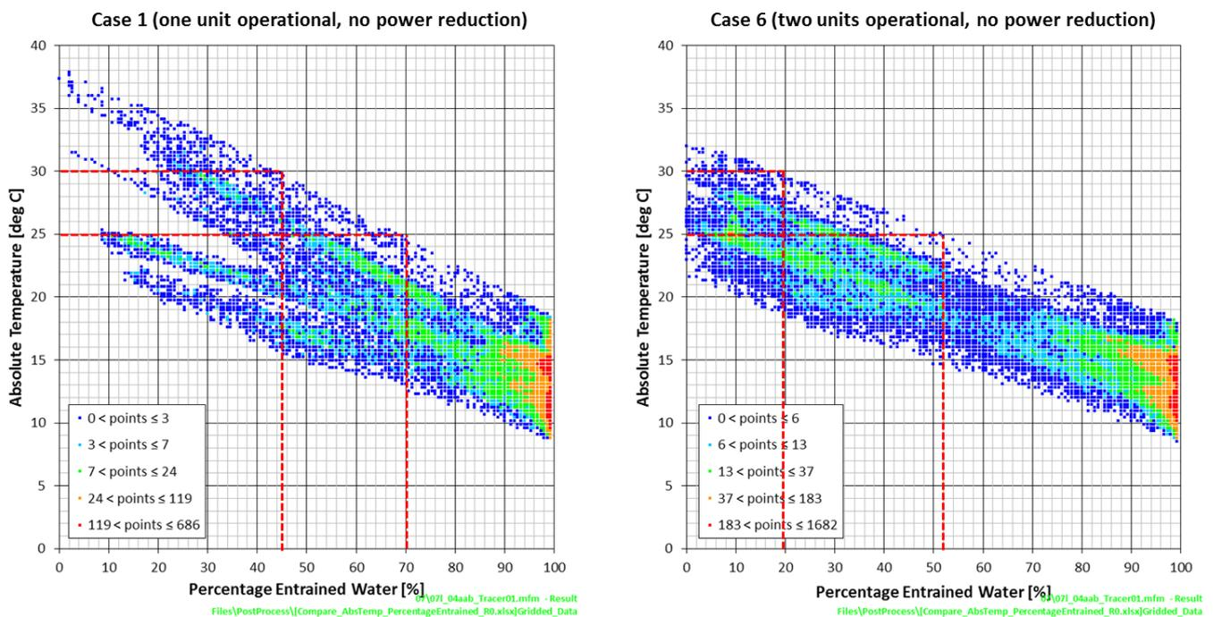
**Figure 4-8: Relationship between absolute temperature and entrainment of ambient seawater for Case 1 (left) and Case 6 (right). 100% entrainment means pure ambient seawater, while 0% entrainment means pure effluent.**
