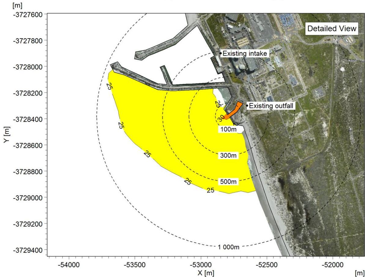
Figure A-7: Maximum absolute temperature near the surface: Case 4 (one unit operational, 50% power).
