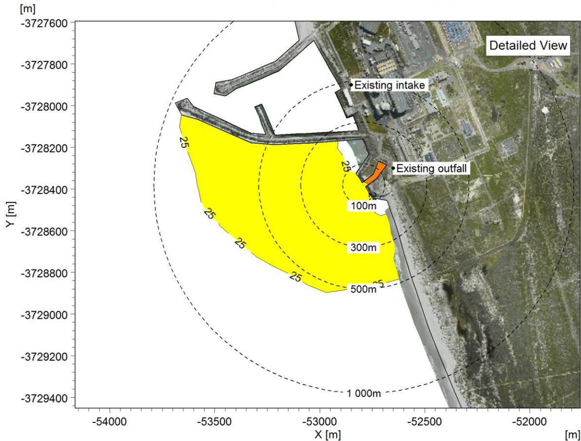
Figure A-9: Maximum absolute temperature near the surface: Case 5 (one unit operational, 40% power).
