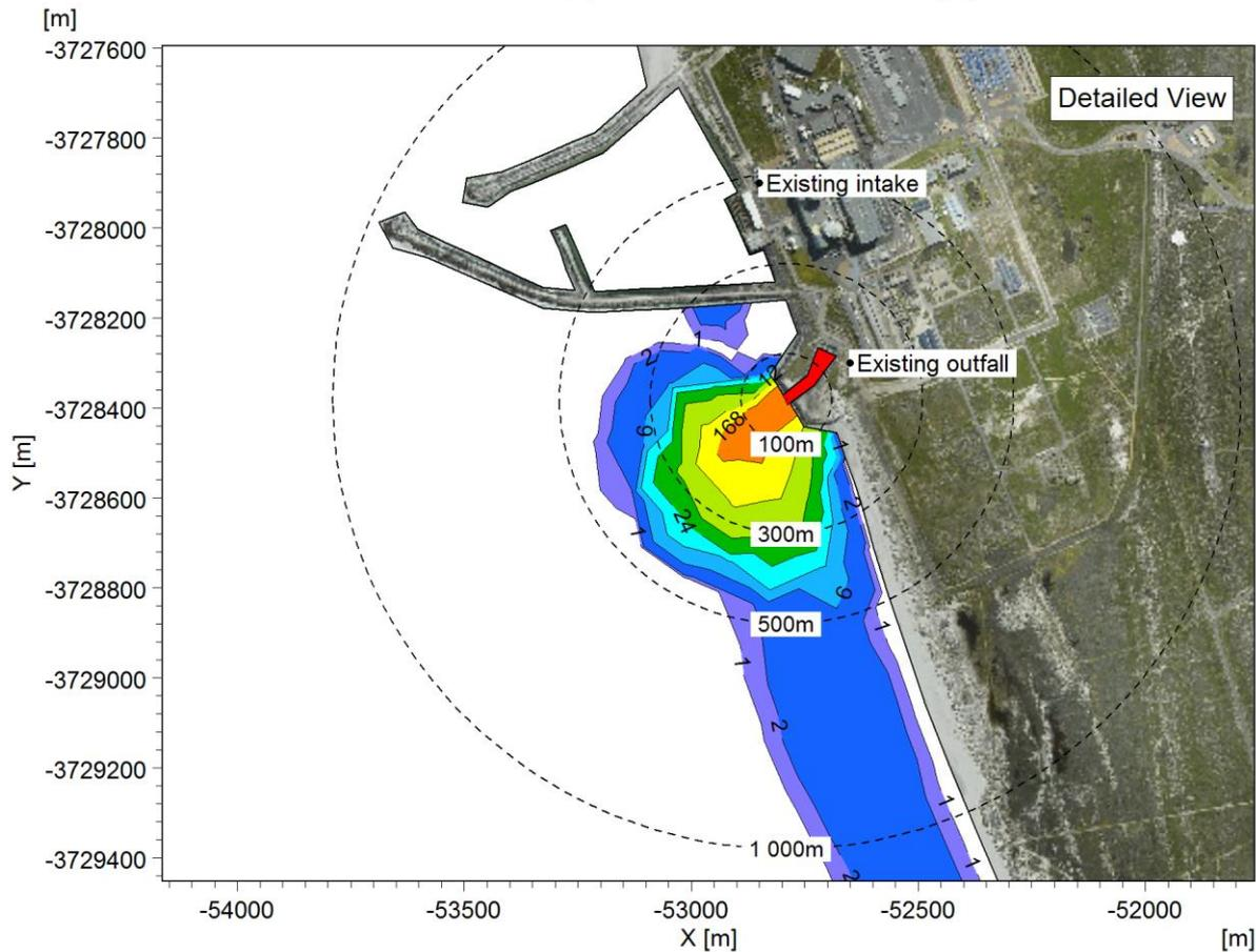
**Figure A-28: Duration that the chronic threshold of 25°C is exceeded near the seabed: Case 7 (two units operational, 70% power).**
