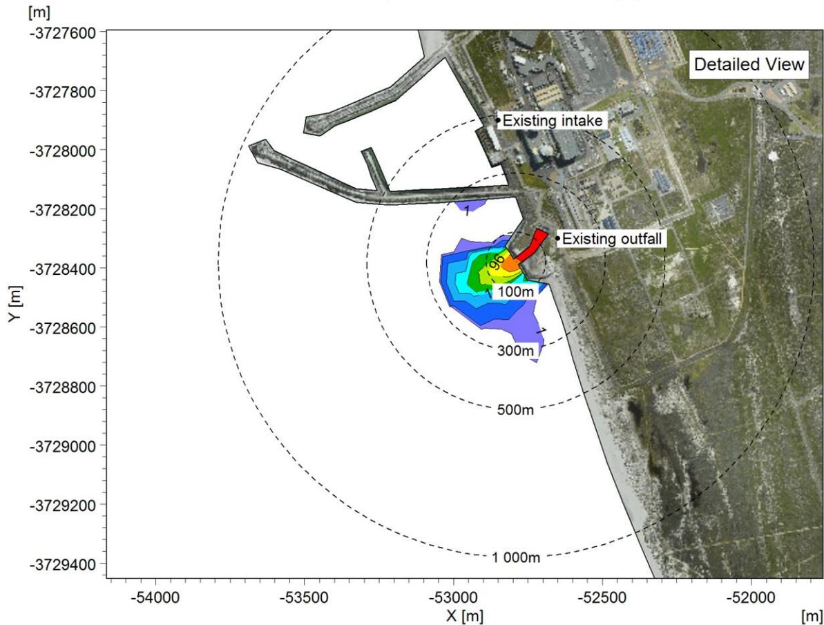
Figure A-22: Duration that the chronic threshold of 25°C is exceeded near the seabed: Case 4 (one unit operational, 50% power).
