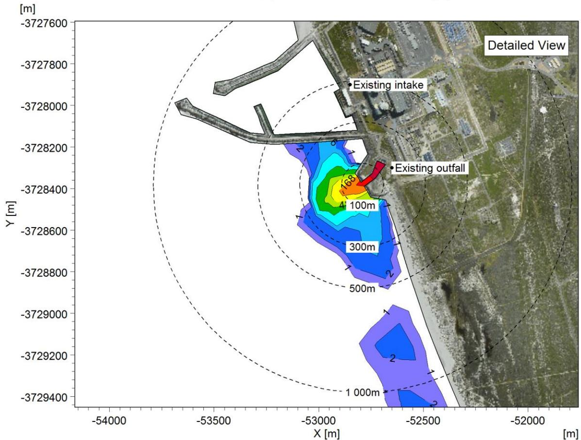
Figure A-16: Duration that the chronic threshold of 25°C is exceeded near the seabed: Case 1 (one unit operational, 100% power).
