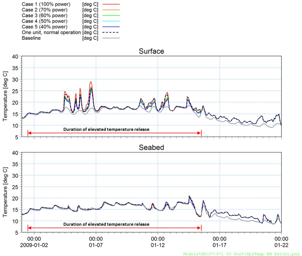
**Figure 4-7: Time series of absolute temperature at the breakwater output location. Cases 1 to 5, seabed and surface.**
