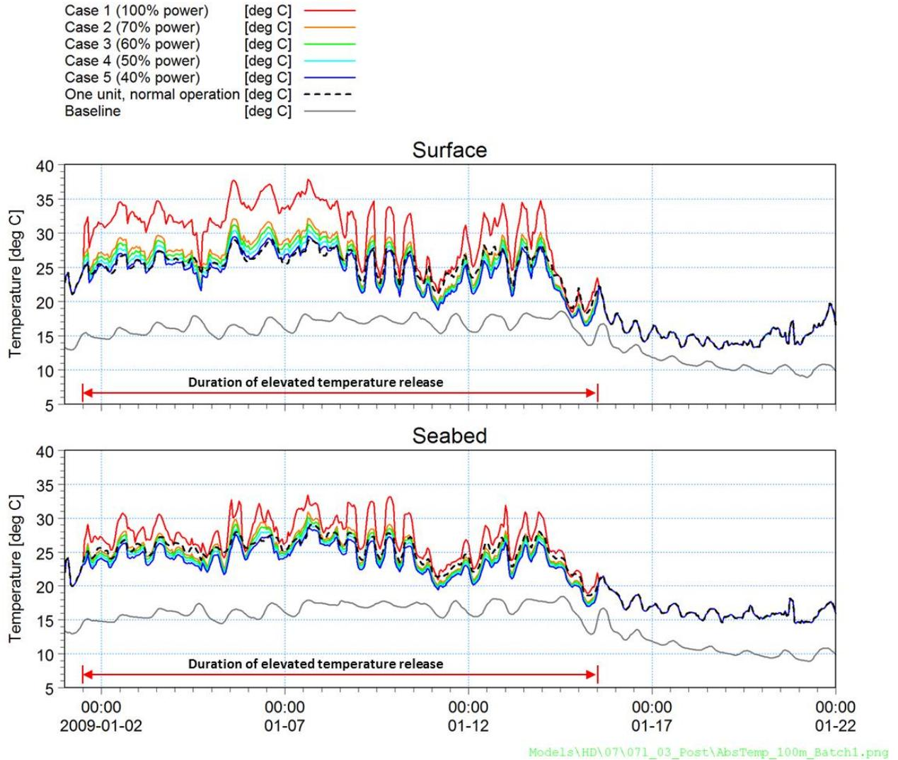
Figure 4-6: Time series of absolute temperature at 100 m from the discharge. Cases 1 to 5, seabed and surface.
