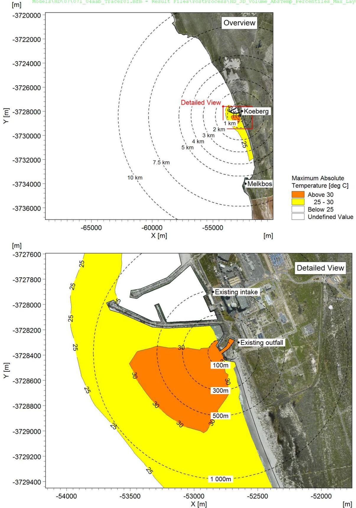
Figure A-11: Maximum absolute temperature near the surface: Case 6 (two units operational, 100% power).
