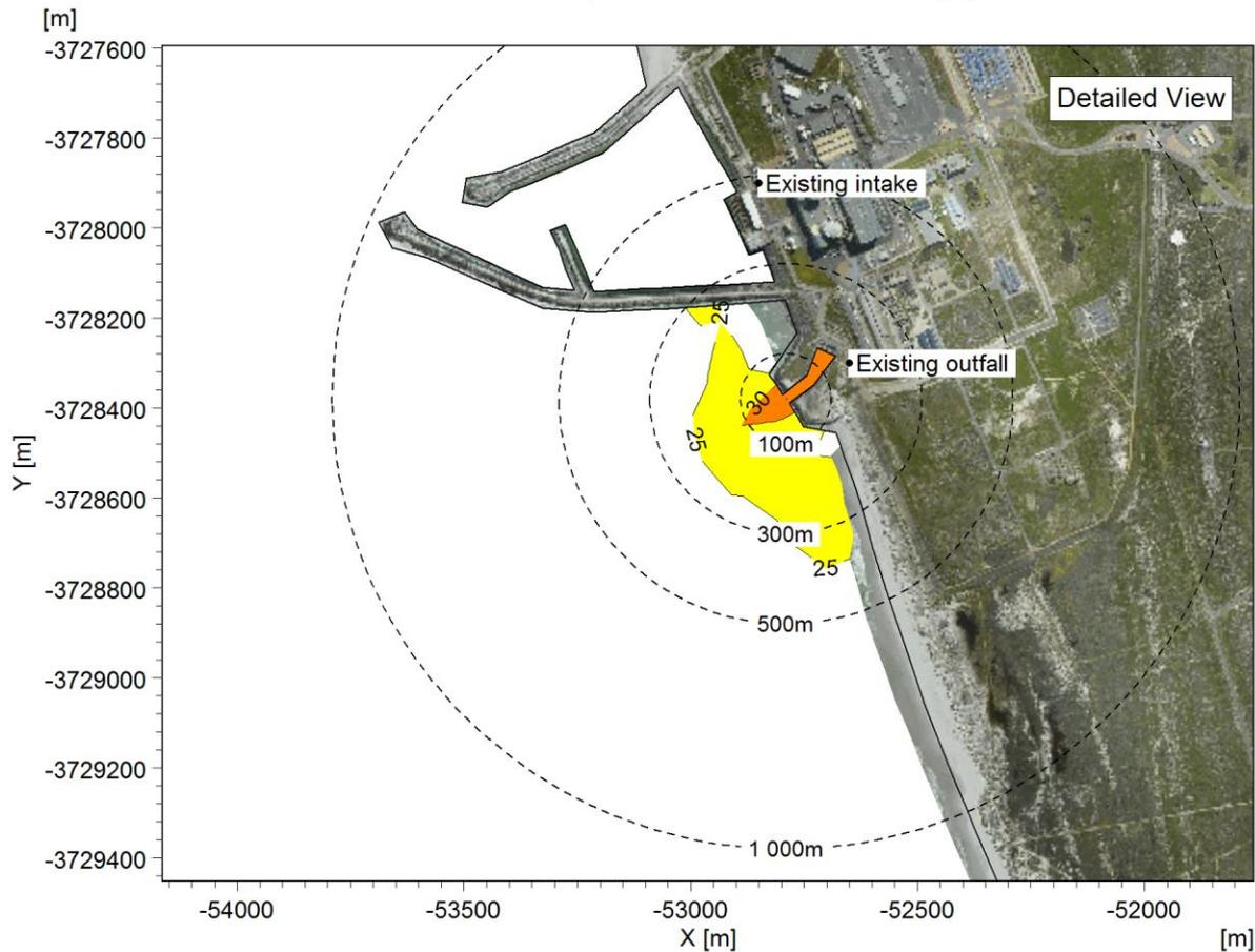
Figure A-4: Maximum absolute temperature near the seabed: Case 2 (one unit operational, 70% power).
