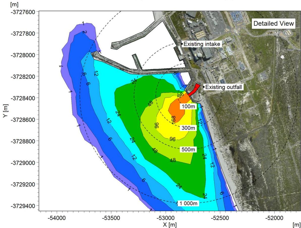
**Figure A-27: Duration that the chronic threshold of 25°C is exceeded near the surface: Case 7 (two units operational, 70% power).**
