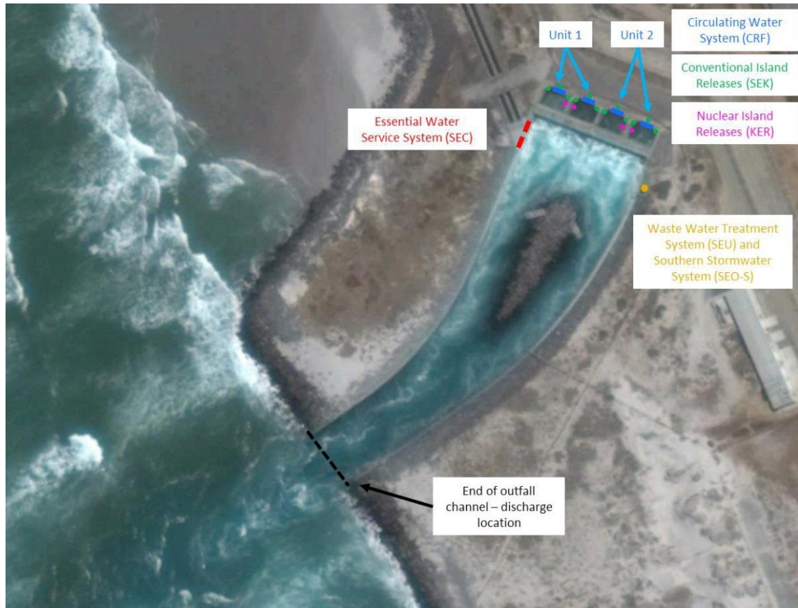
Figure 4: Layout of effluent streams released into the KCWOB (source: PRDW, 2017)
