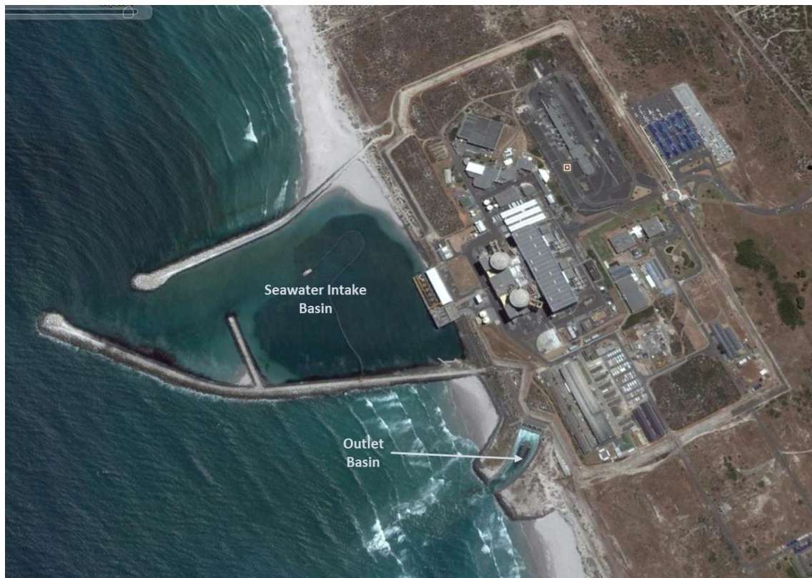
Figure 1.1: Google Earth view of the KNPS and discharge on the Cape west coast. Seawater from the intake basin is pumped through the power plant and discharged into the outlet basin. Discharge jet momentum can be high allowing the discharge plume to cross the surf zone.
