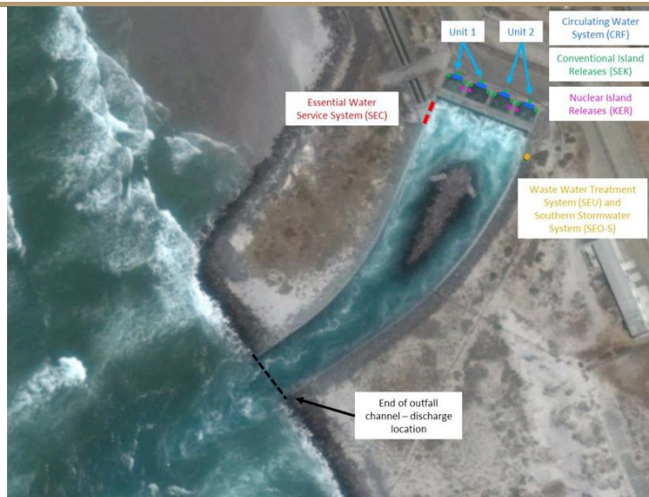
Figure 1: Layout of effluent streams released into the KCWOB (source: PRDW, 2016)
