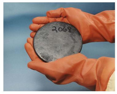
In order to sustain fission chain reaction, the uranium is processed in an enrichment facility to increase the concentration of isotopes to 4.4% for use at Koeberg.
