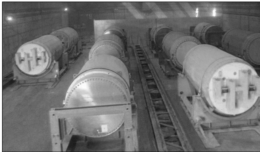
Umfanekiso 22: Imigqomo yokugcina amafutha ekufakwa kuyo ii-assembly zamafutha enyukliya
