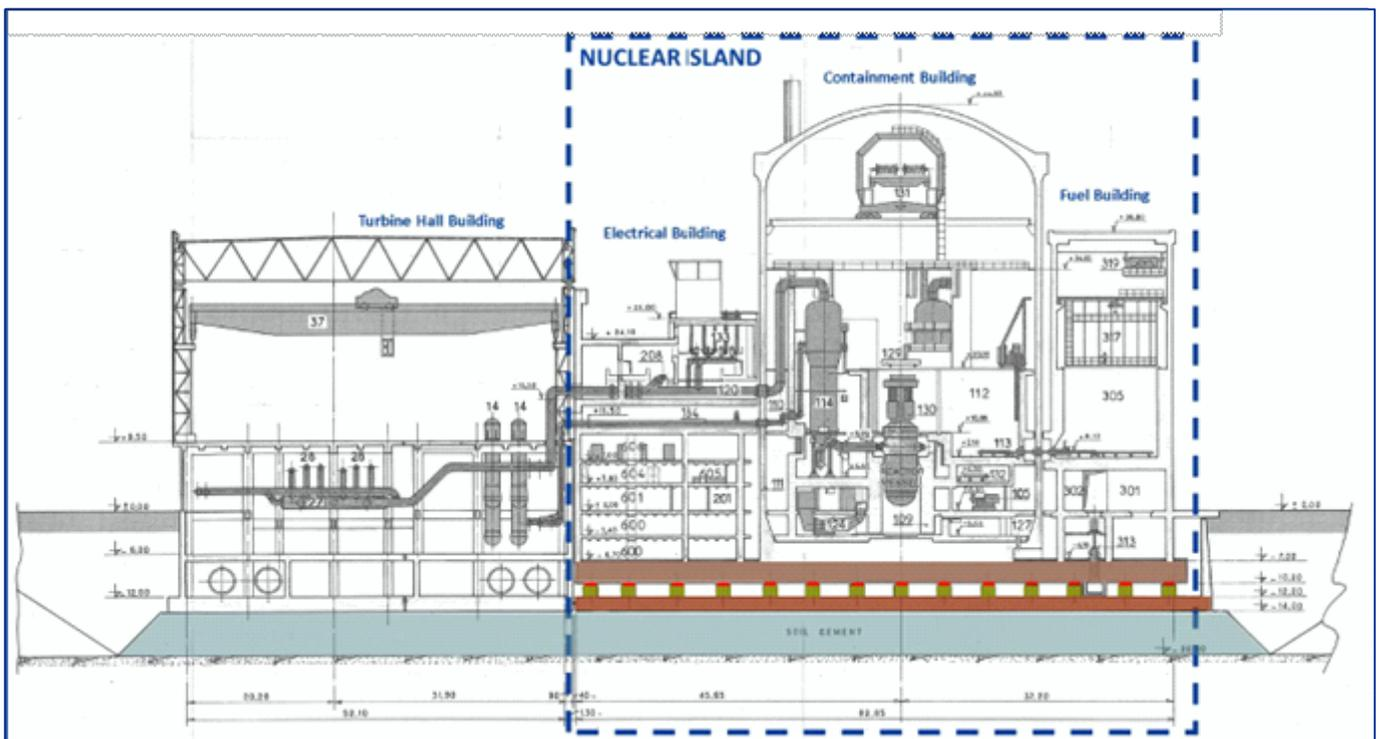
Figure 1: Overview of KNPS Main Plant
