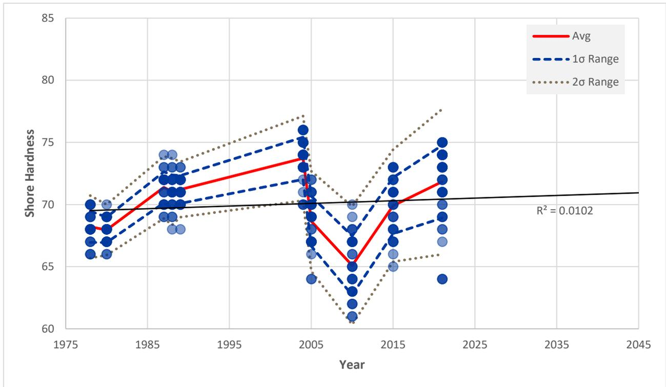
**Figure 12: Shore Hardness Values from Monitoring Programme**
