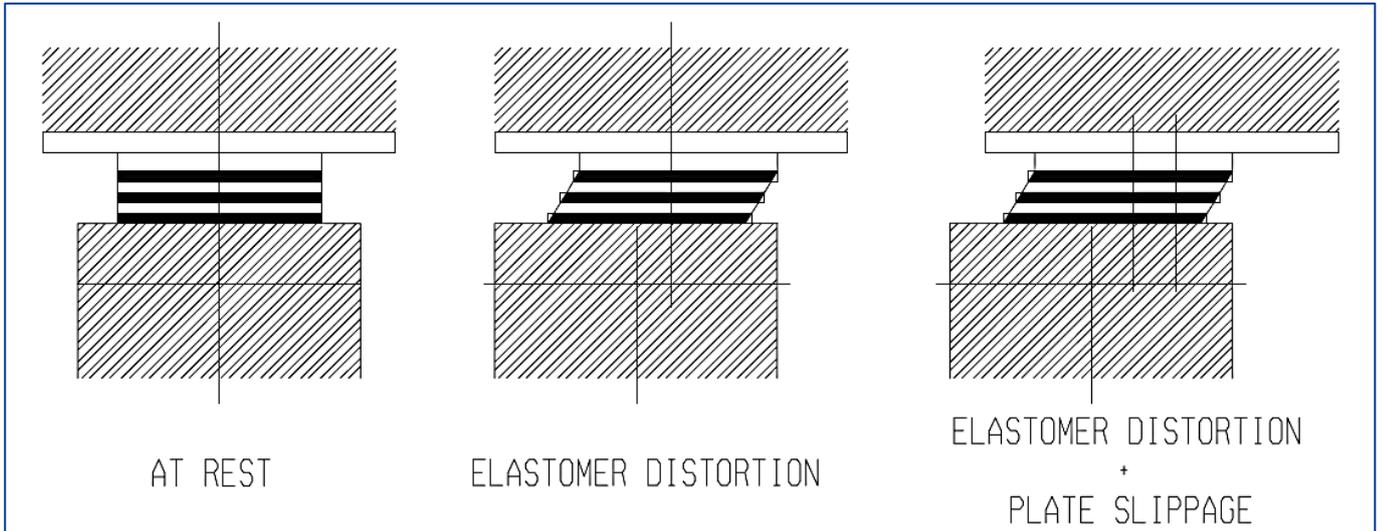
**Figure 10: Dynamic Behaviour of the Aseismic Bearings**
