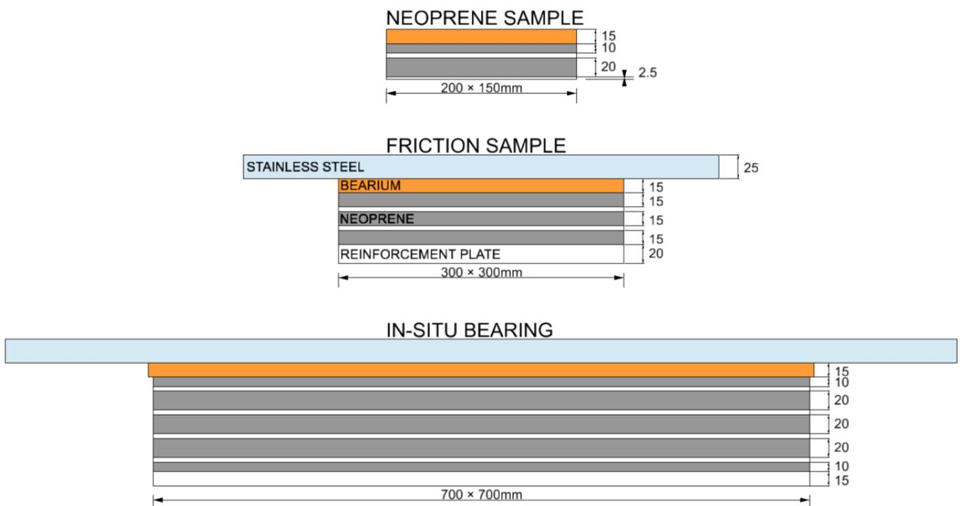
Figure 6: Overview of Samples and In-Situ Bearings Composition
