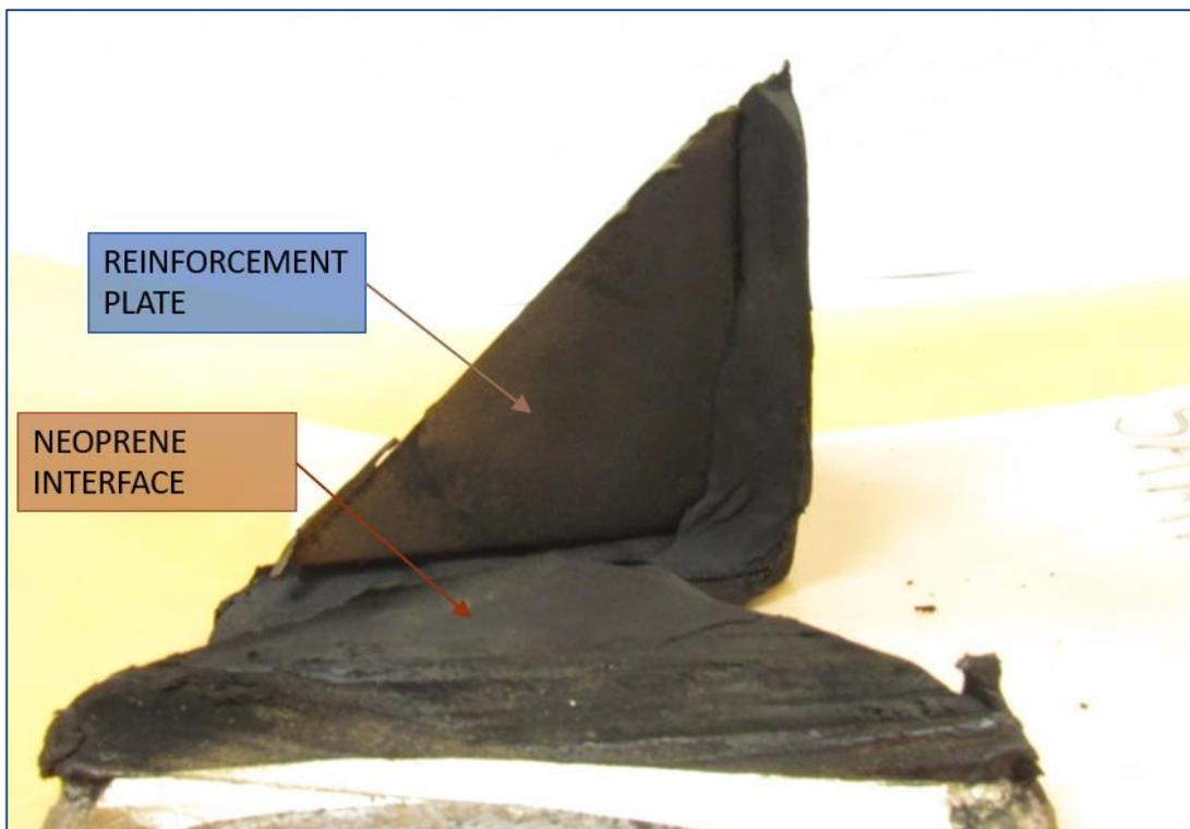
**Figure 11: Broken Bond between Reinforcement Plate and Neoprene**
