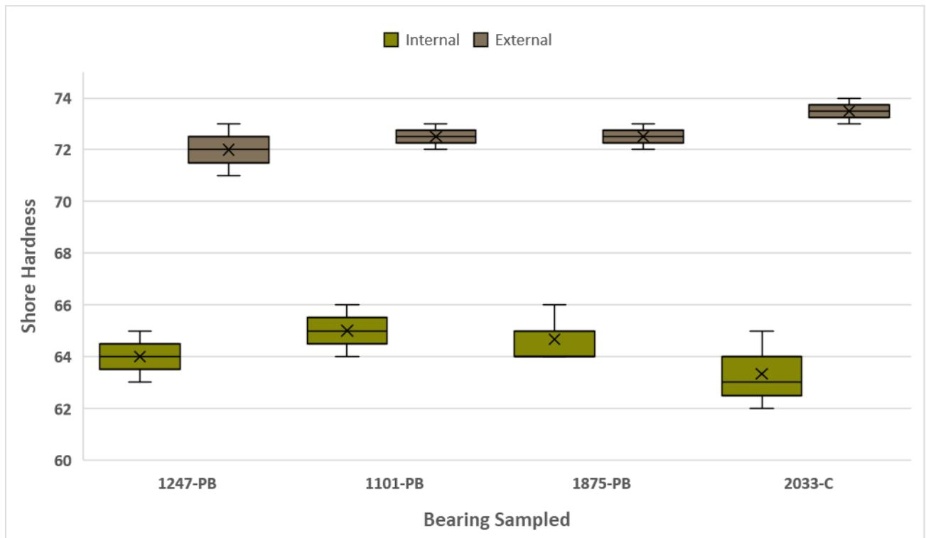
**Figure 15: Internal vs. External Shore Hardness Measurements**
