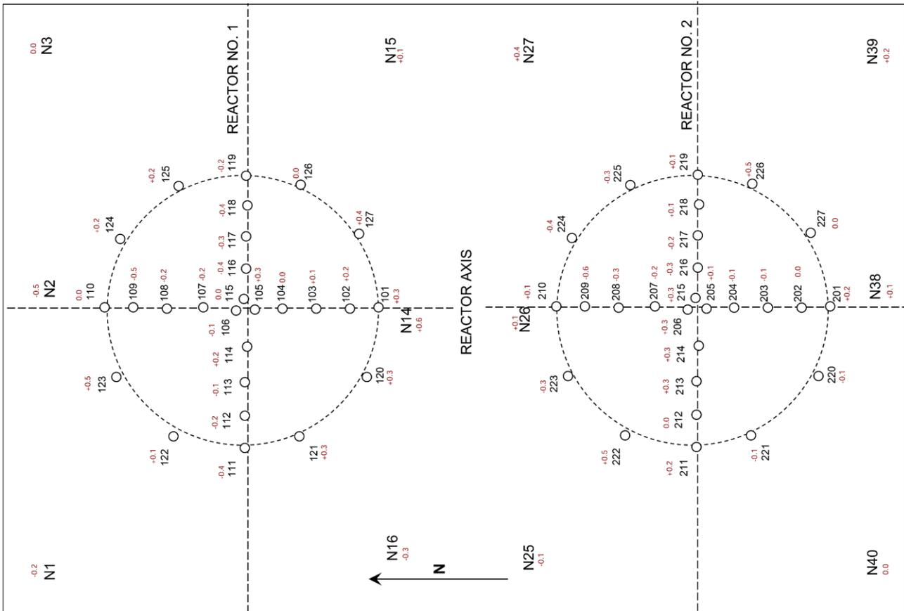
**Figure 7: Aseismic Vault - Relative height differences in millimetres, 2021-2016**
