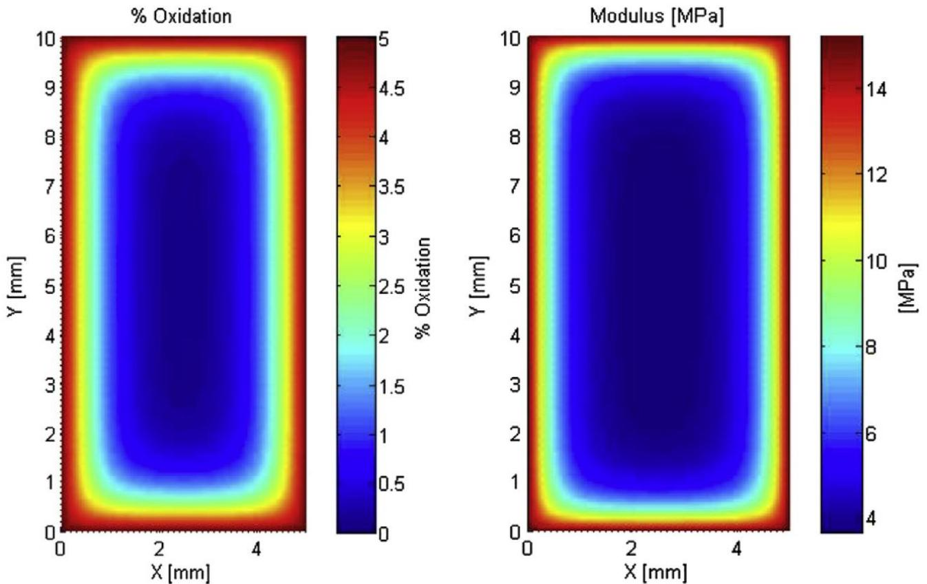
**Figure 14: Diffusion limited oxidation and its predicted correlation with localized modulus for a neoprene elastomer<sup>6</sup>**
