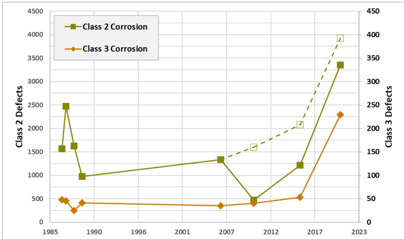
**Figure 24: Corrosion Defects Trending**
