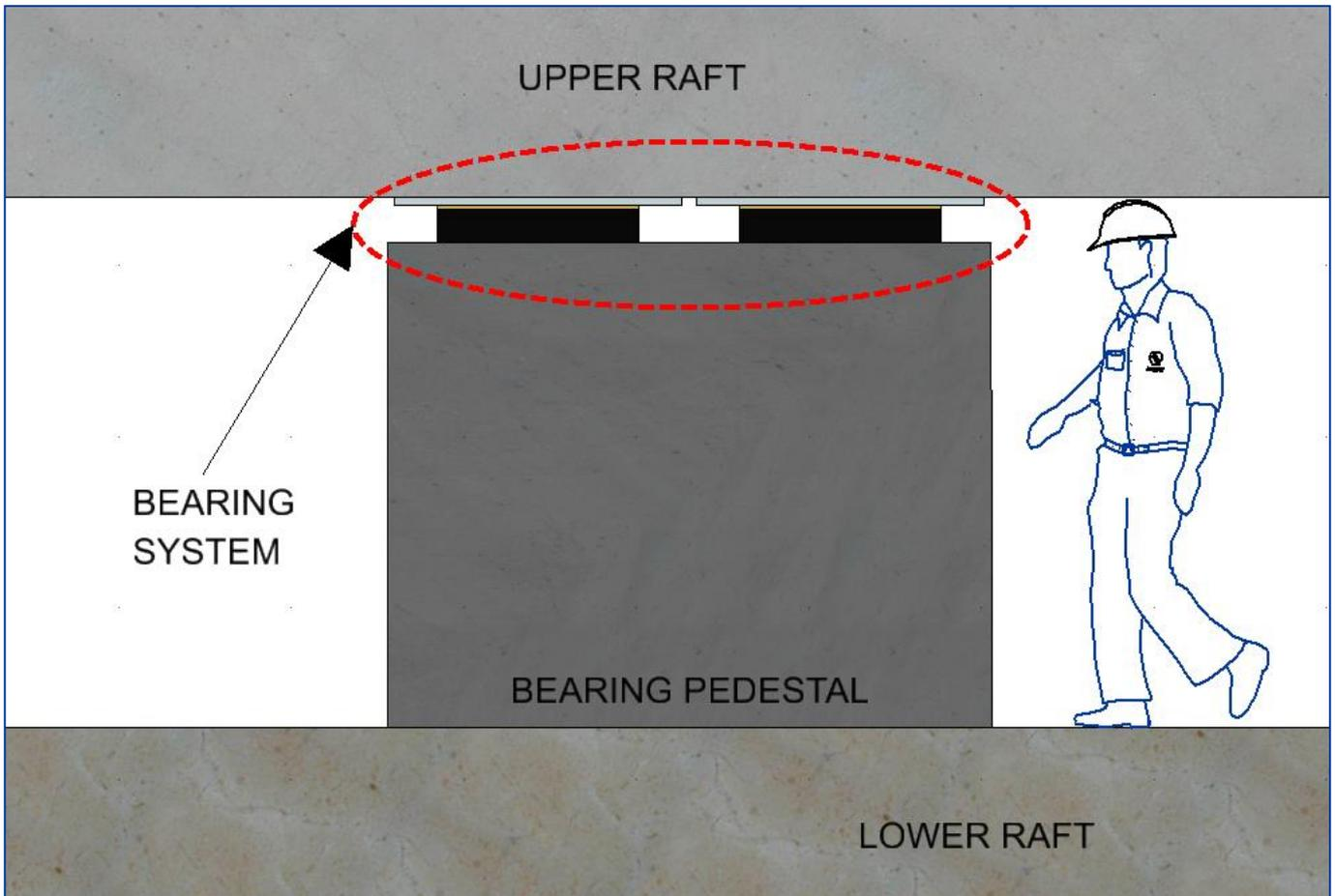
Figure 3: Schematic of Nuclear Island Foundation System
