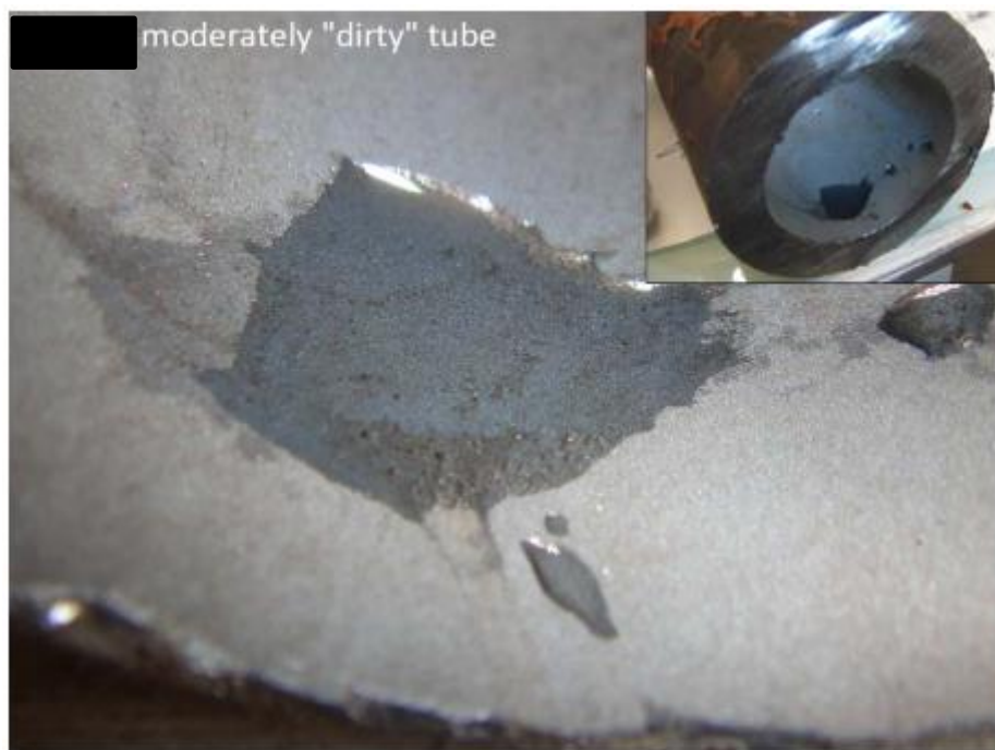
Figure 11: Appearance of a boiler tube with a “poor” hydrophobic coating.
