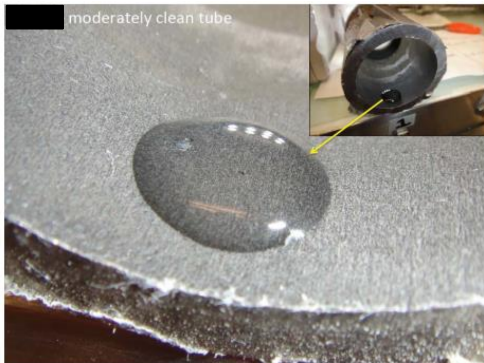
Figure 10: Appearance of a boiler tube with a “moderate” hydrophobic coating.
