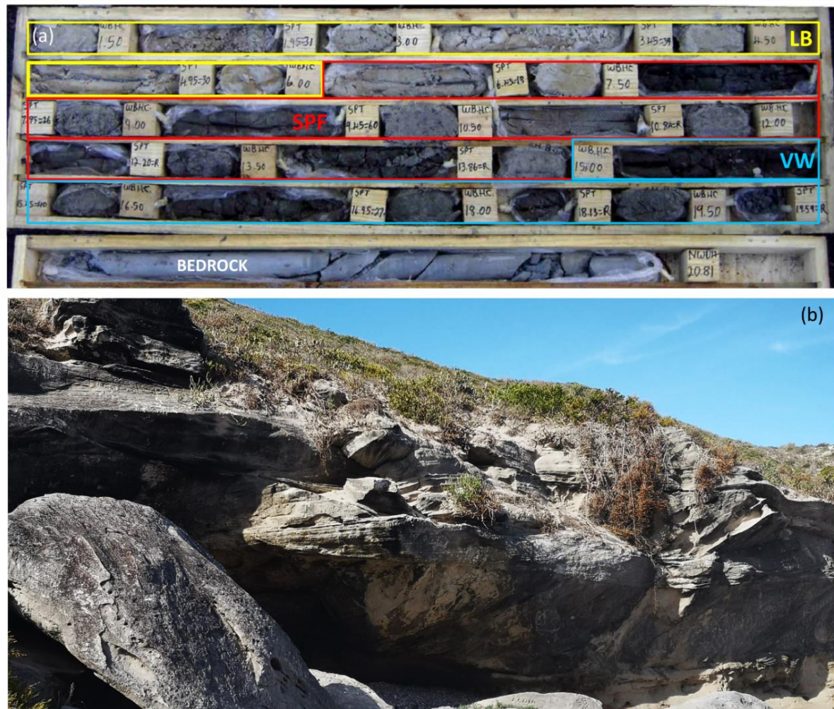
Figure 4-44. Langebaan Formation sediments encountered (a) in borehole BH8 (Day and Ridgway, 2000) at the Duynefontyn site between 0-6 m depth, and (b) exposures of cross-bedded aeolianite south of Tieties Baai (S 32°50'30.68"; E 17°51'55.83").
