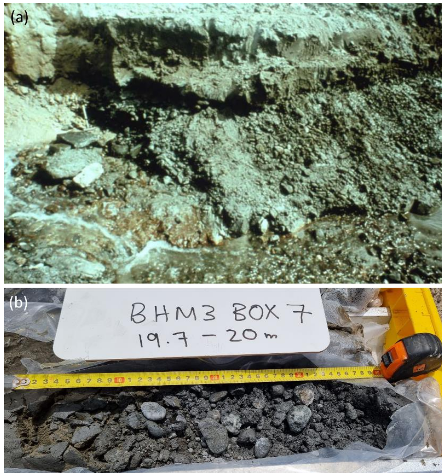
Figure 4-41. (a) Basal gravels of the Silwerstroom Member (Varswater Formation) that correlates to the ‘Basal Gravel bed’ first identified by Rogers (1979) during excavations at Koeberg and (b) at Duynefontyn in borehole M3 at a depth of 19.7-20 m (Claassen et al., 2023).
