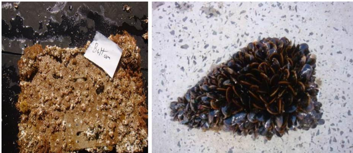
Figure 5.9.155: Biofouling after 6 Months at 8 m Depth (Left) and After 14 Months in 10 m Depth (Right).
