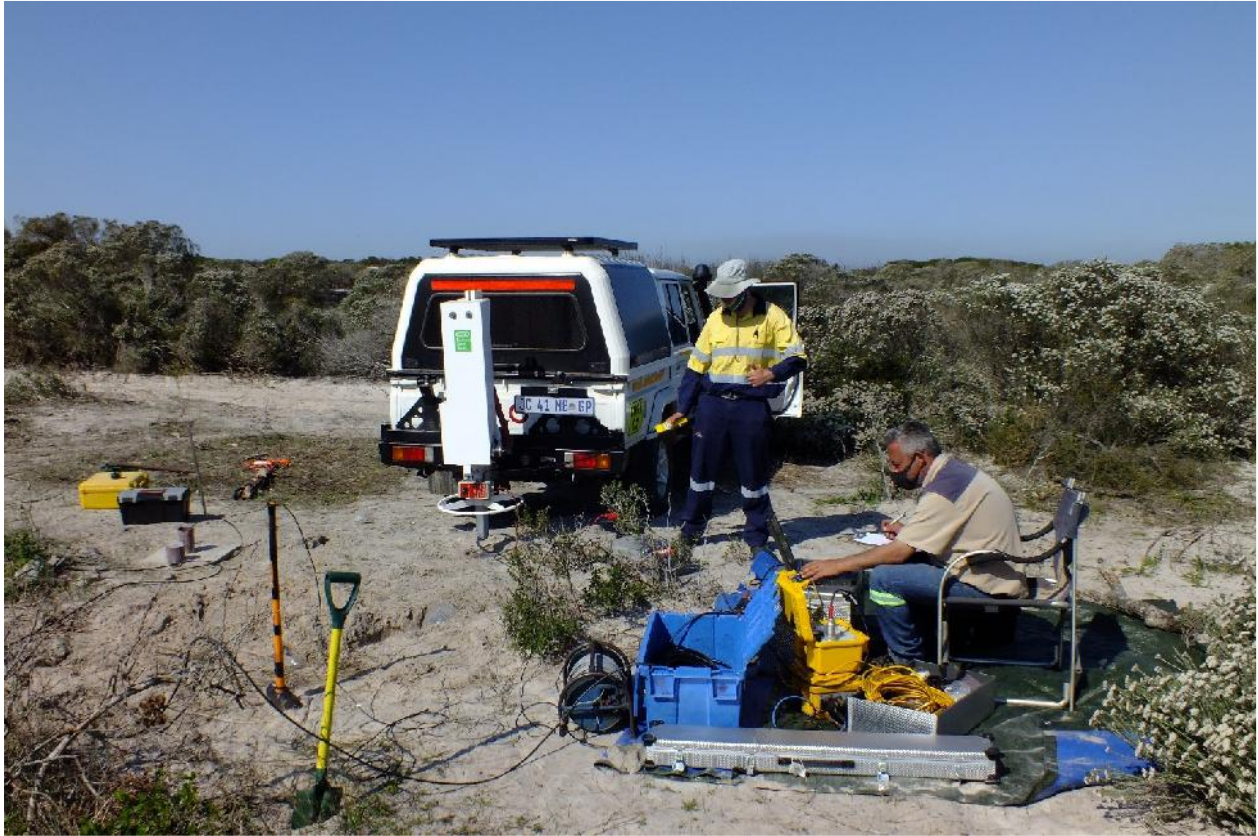
Figure 5. Downhole Seismic Survey at BH47
