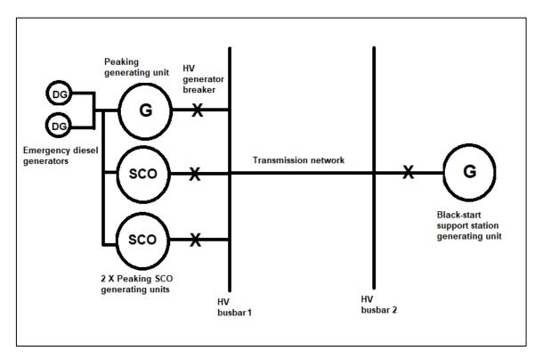
Figure 2 - Example of a partial black-start test network for a peaking black-start facility
