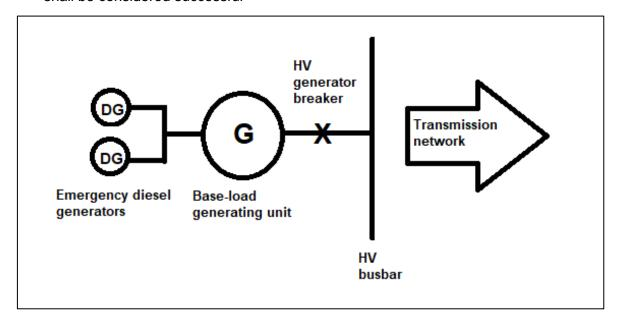
Figure 1 - Example of a partial black-start test network for a base-load black-start facility
