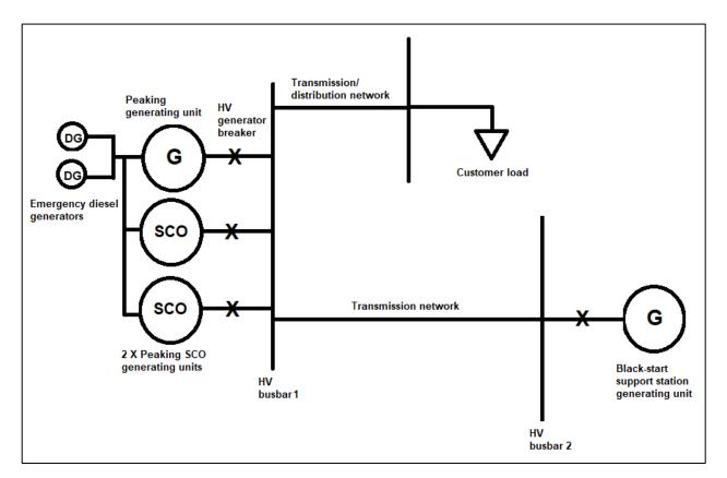
Figure 4 - Example of a full black-start test network for a peaking black-start facility
