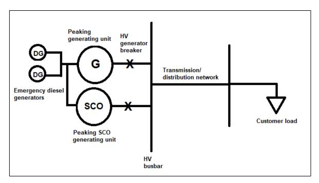
Figure 5 - Example of a routine self-start test network
