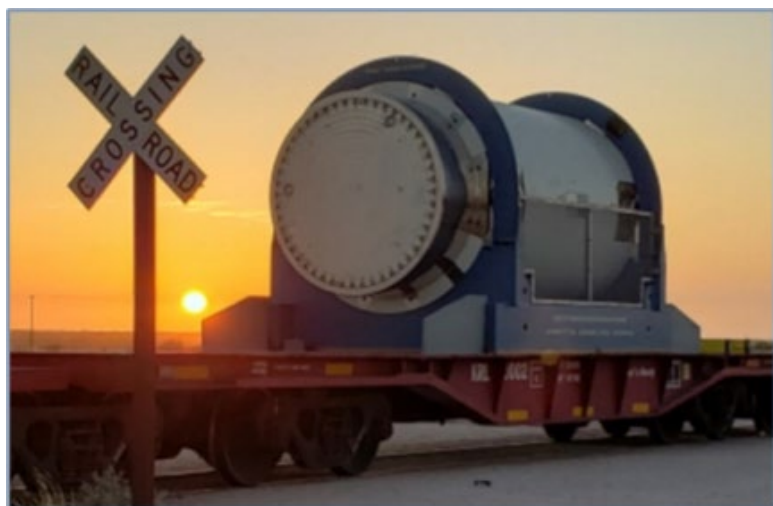
Figure 15: Dry cask for nuclear fuel storage
