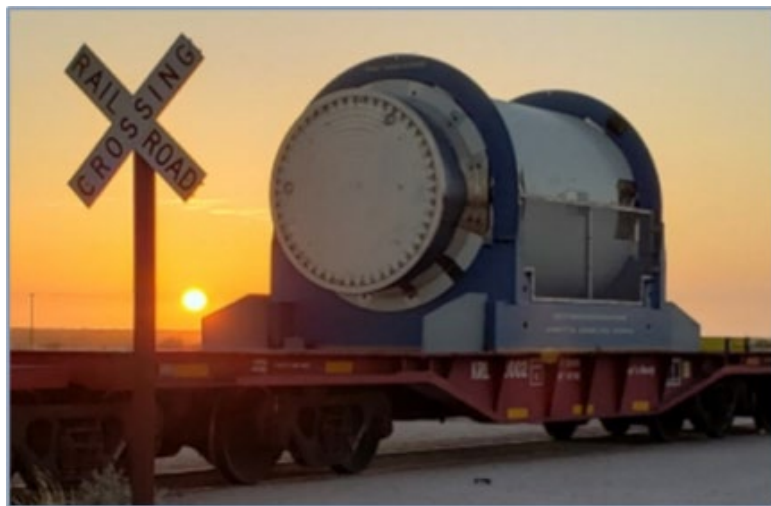
Figure 15: Dry cask for nuclear fuel storage
