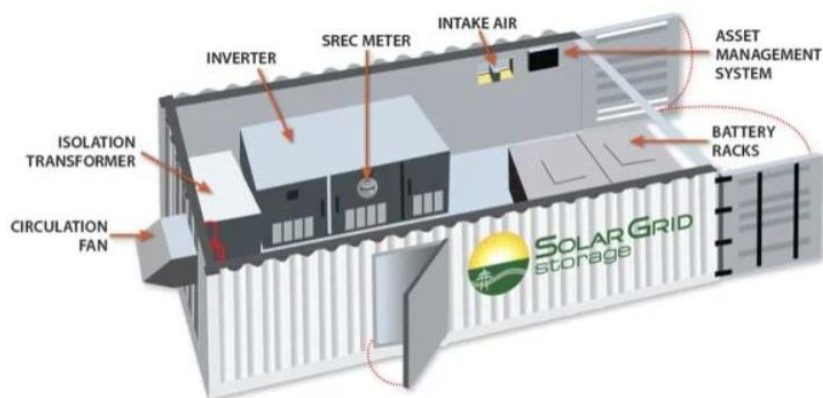
Figure 5-4 – Typical Battery Modules in a BESS with the Separated Sections
