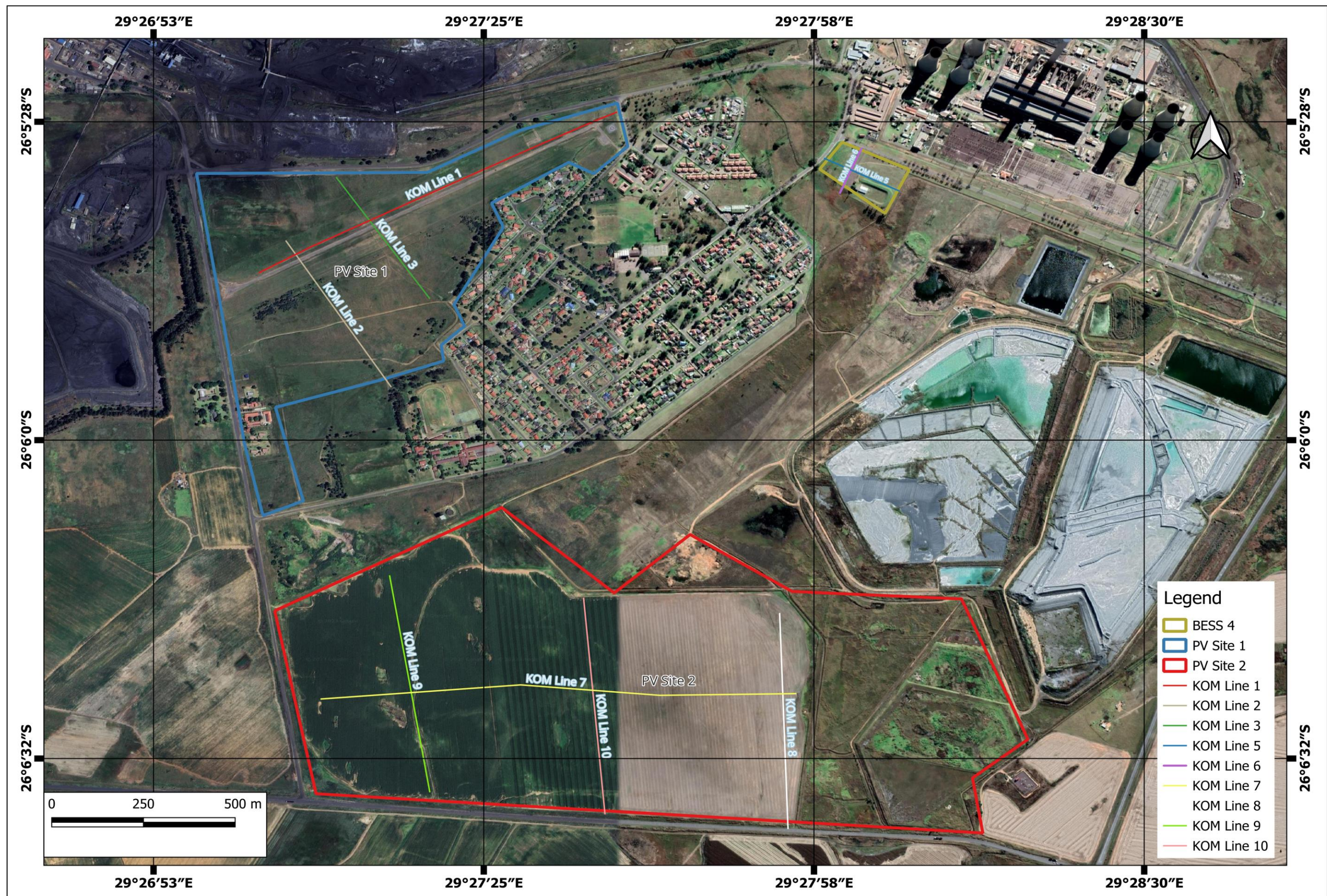
Figure 4-11: Geophysical map showing resistivity survey lines
