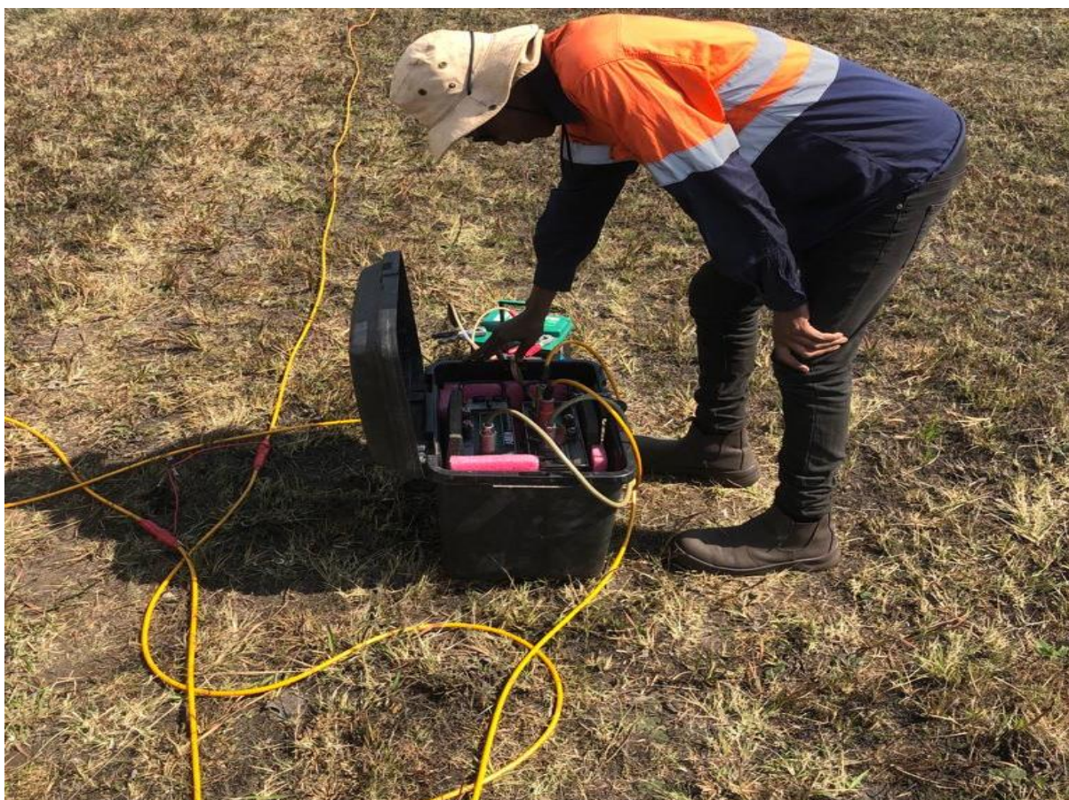
Figure 4-1: Geophysical survey for soil resistivity by means of ABEM terrameter SAS1000.
