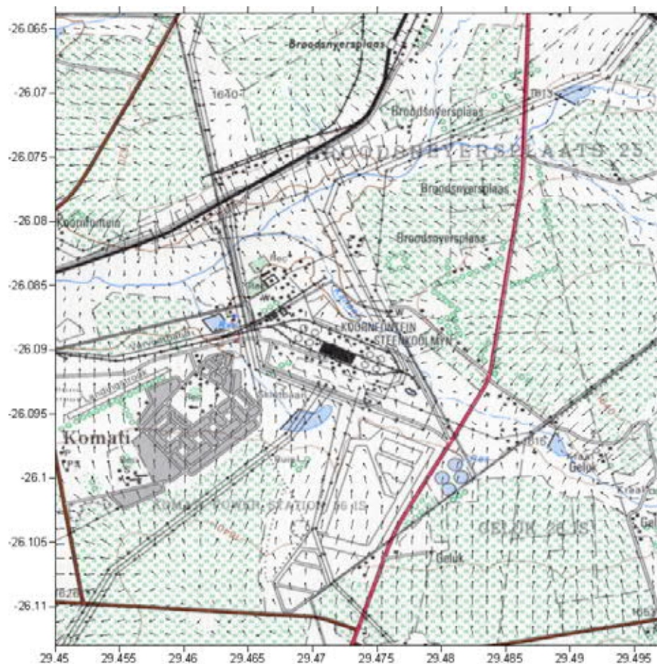
Figure 2. Surface drainage indicating flow directions
