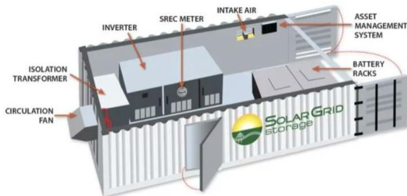
Figure 3-4 – Typical Battery Modules in a BESS with the Separated Sections
