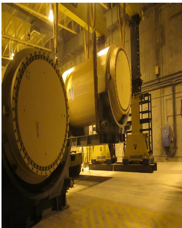
Figure 5: Placement and Storage of Casks in the Koeberg CSB
