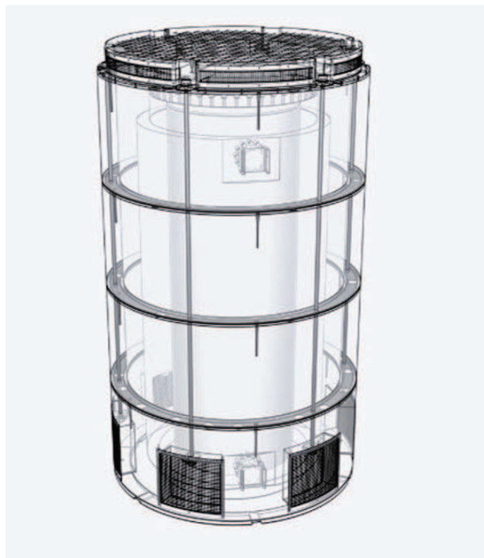
Figure 15: Vertical Auxiliary Shielding Module (MAB) for Metallic Cask ENUN 52B
