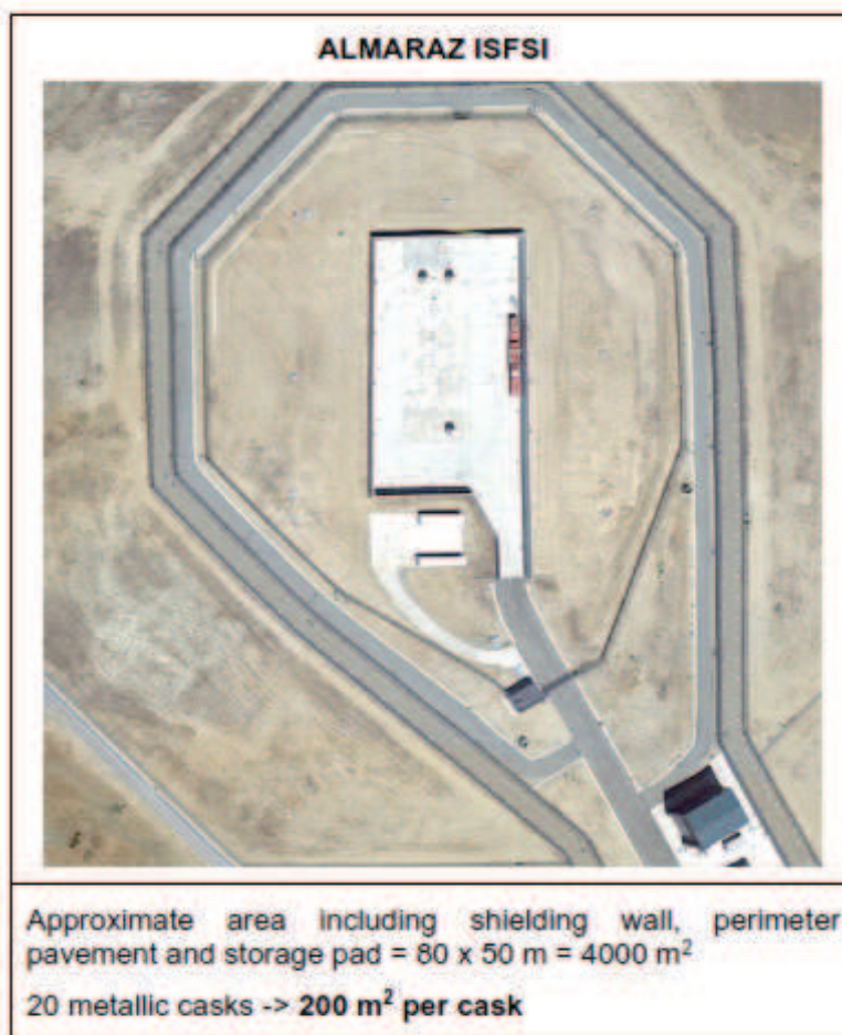
Figure 17: ISFSIs Footprint with Metallic Casks – Almaraz ISFSI
