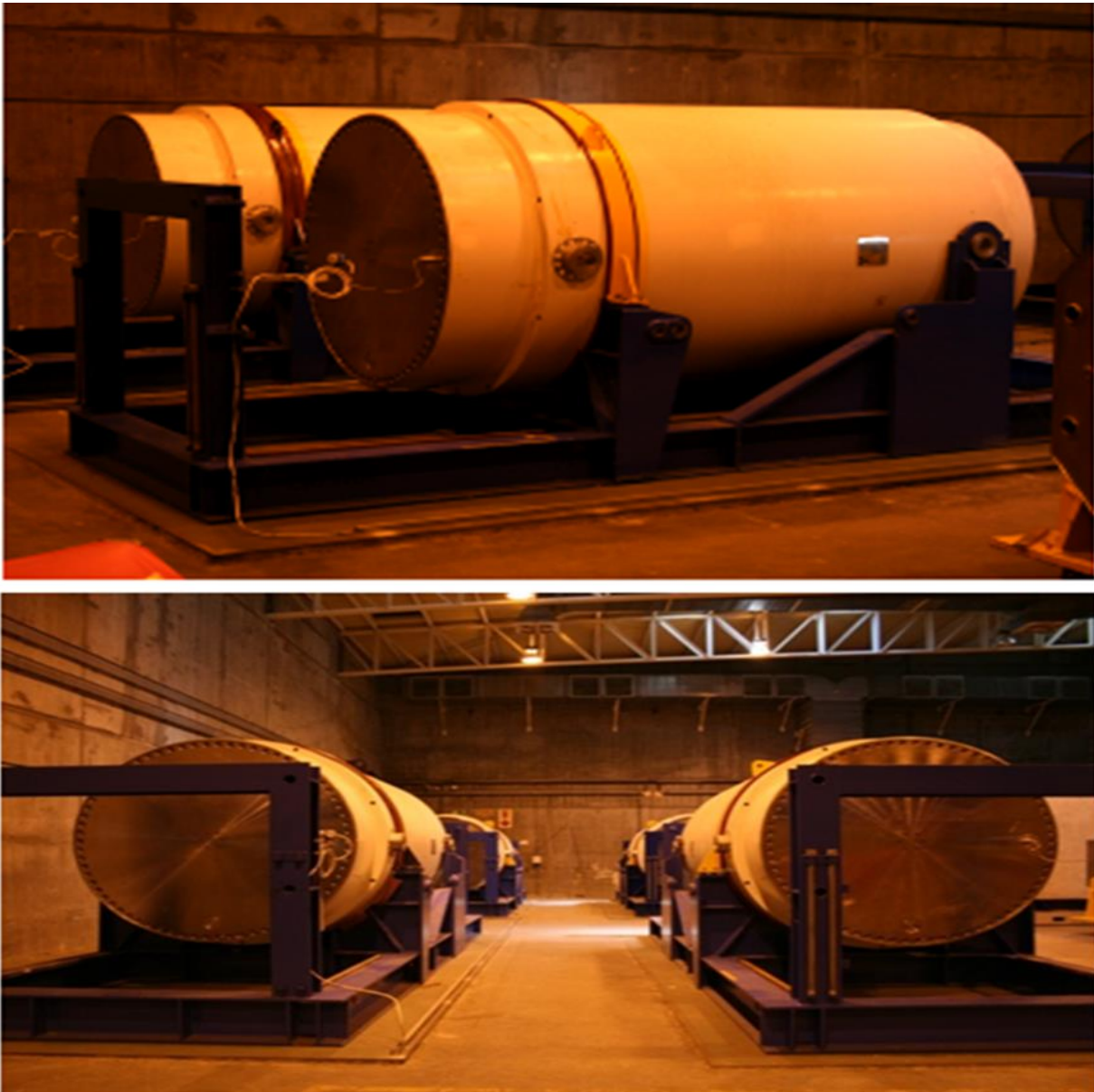
Figure 2: CASTOR X /28F Cask Storage in the Koeberg CSB
