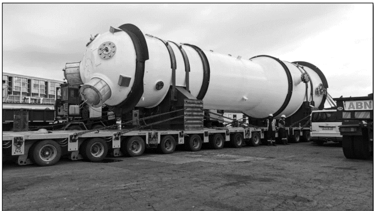
Figure 3: The new Koeberg steam generators being delivered in South Africa
