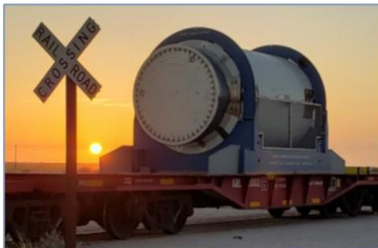
Figure 14: Dry cask for nuclear fuel storage
